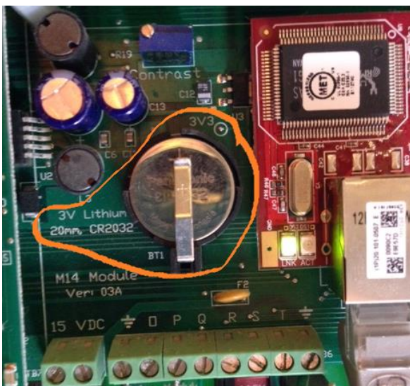
Battery with holding arm in MultiFLEX controller
