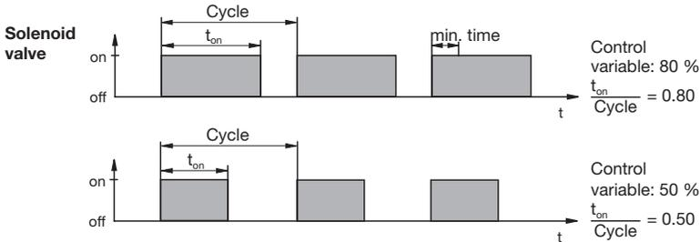
The switching time of the DULCOMETER® D1C (solenoid valve) depends on the control variable and the “min. time” (smallest permitted operating factor of the connected device).
