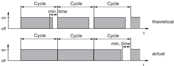
The DULCOMETER® D1C does not deactivate for a certain number of cycles until the differences between cycle and theoretical switching time exceed the “min. time”.
