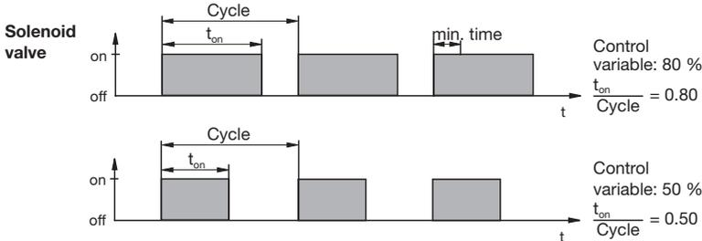
The switching time of the DULCOMETER® D1C (solenoid valve) depends on the actuating variable and the “min. time” (smallest permitted operating factor of the connected device).
