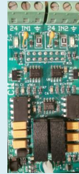
The long distance transmitter uses 2 conductor cable, 18 to 22AWG
