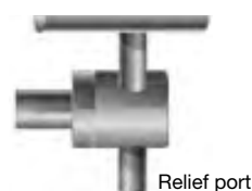
Backpressure valve on tee for pressure relief
