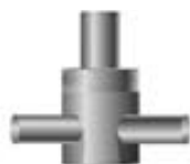
Backpressure valve (2 port)
