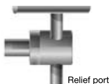
Backpressure valve on tee for pressure relief
