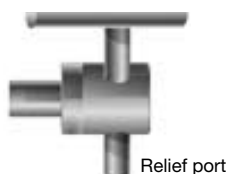
Backpressure valve on tee for pressure relief
