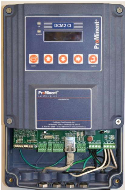
Interior of DCM 200 controller
