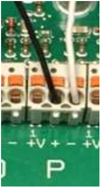
Figure 34 Digital Input wiring
