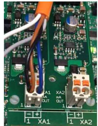
Figure 60 Dual mA Output with ProMinent Universal Control Cable on output 1.
