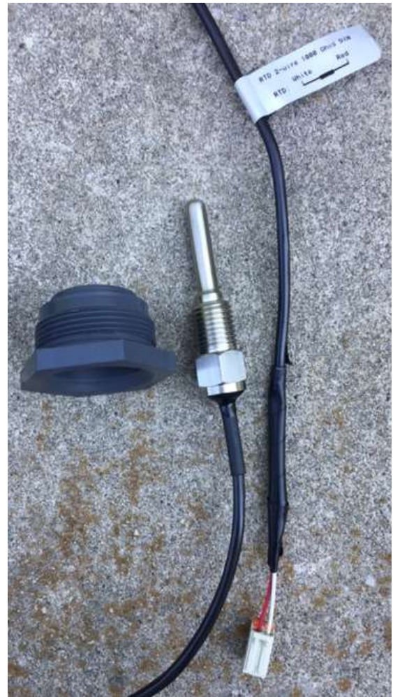
Figure 5 PT1000 Black cable 2 wire temperature sensor with DGMa adapter
