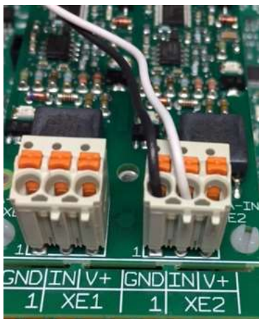
Figure 57 Two wire remotely powered analog input
