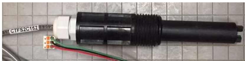
Figure 38B CTFS sensor shown without adapter
