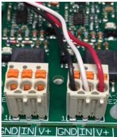
Figure 56 Three wire 4-20mA inputs that utilize V+
