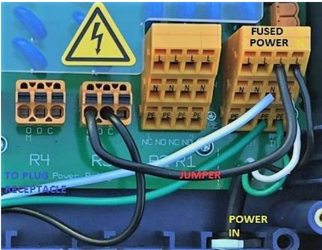
Figure 25 Wiring R3 using on-board fused power
