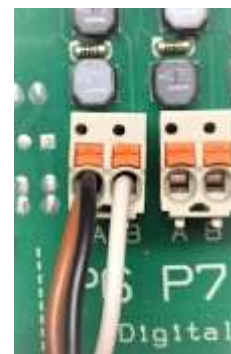
Figure 29B Universal Control Cable on Output Relay P6 (Pulse Mode)
