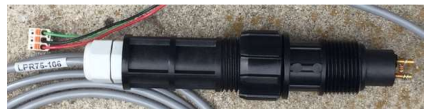
Figure 38A Corrosion rate LPR serial sensor (Linear Polarization Resistance) Shown with test resistor and adapter
