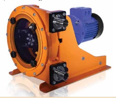
The **DulcoFlex DFC** is a hose pump designed for difficult pumping applications. Unlike typical shoe pumps, it incorporates a roller design, which eliminates the need for cumbersome lubricants. The **DFC** can reach pressures up to **116 psi** and flow rates up to **106 gpm** and is ideal for difficult industrial and municipal applications.
