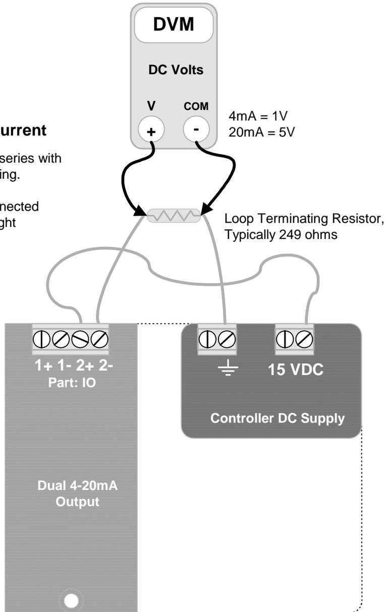
Hardware Calibration is used to compensate for component level errors. It's only available via the keypad and forces the current loop to 20mA to adjust SPAN and to 4mA to adjust ZERO. Trim Zero default = 9 Trim Span default = 950
