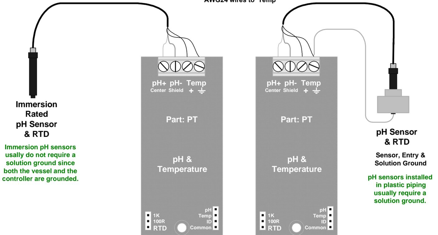
At temperatures below 75F / 25C, higher internal pH impedance limits a pH sensor's cabling to nominally 25ft or 10m.
