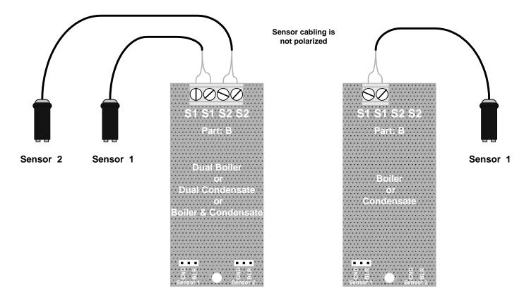
Conductivity sensor cabling may be extended up to 200ft / 60m, using single pair AWG22 / 0.25 mm<sup>2</sup>, cable spliced to the sensor cable using wire nuts or crimped connectors located in an electrical fitting or enclosure.
