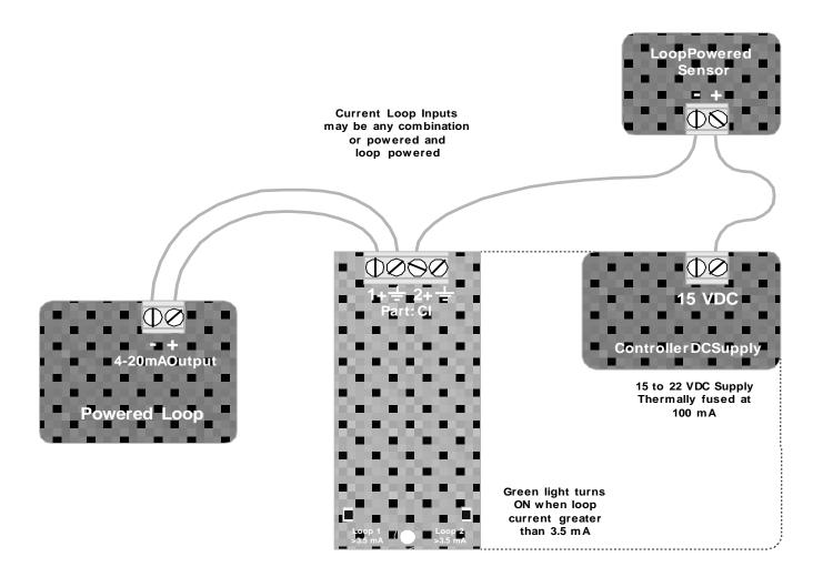
$AWG22 / 0.25 \text{ mm}^2$ , current loop cabling may be extended several hundred feet or meters without causing measurement errors. The maximum cable length is determined by the open loop voltage and the cable gauge.
