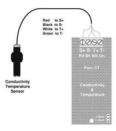
Conductivity sensor cabling may be extended up to 200ft / 60m, using two pair AWG22 / 0.25 mm<sup>2</sup>, cable spliced to the sensor cable using wire nuts or crimped connectors located in an electrical fitting or enclosure.
