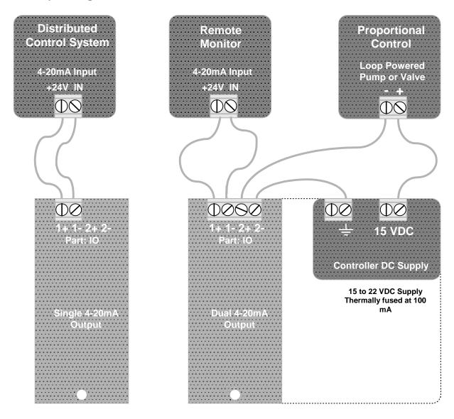
AWG22 / 0.25 mm², current loop cabling may be extended several hundred feet or meters without causing measurement errors. The maximum cable length is determined by the open loop voltage and the cable gauge.
