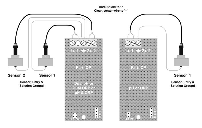
ORP sensor cabling may be extended up to 200ft / 60m, using single pair AWG22 / 0.25 mm², cable spliced to the sensor cable using wire nuts or crimped connectors located in an electrical fitting or enclosure. Higher internal impedance pH sensor's cabling cannot be extended more than 25ft, 10m.
