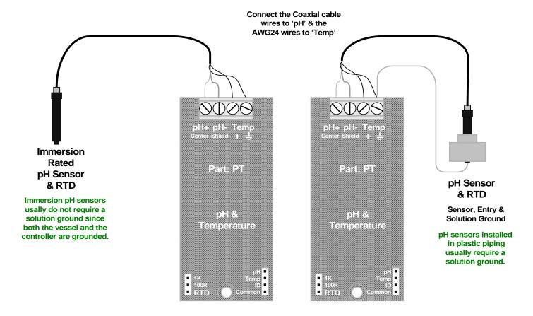
At temperatures below 75F / 25C, higher internal pH impedance limits a pH sensor's cabling to nominally 25ft or 10m.
