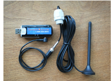
Picture of corded antenna connected to the USB modem (water-proof enclosures are designed for field addition of corded antennas).
