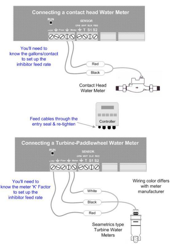
Do not install meter cabling in the same conduit at AC power wiring.
