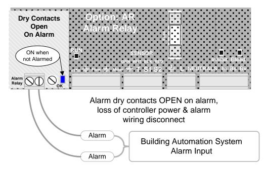
Wire alarm contacts AWG22 to AWG18, 2 conductor
