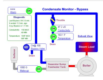
Measures Conductivity, Temperature, Make-up Water Meter and Operating Interlock
