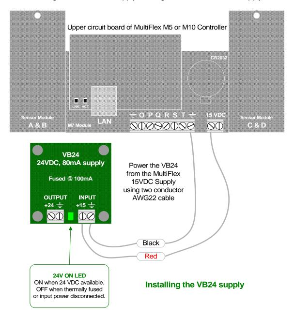
The VB24 is supplied pre-wired to the controller 15VDC power as shown in the previous graphic. It is installed on the backplate at the right bottom of the controller enclosure below the power-relay circuit board.
