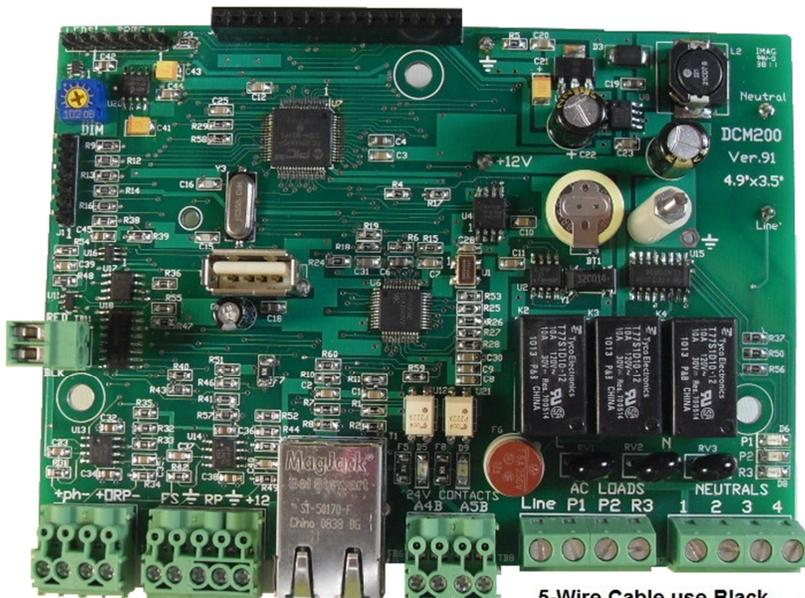
Pulse outputs connect to 'External Control' input requiring a low current DC switch closure.
