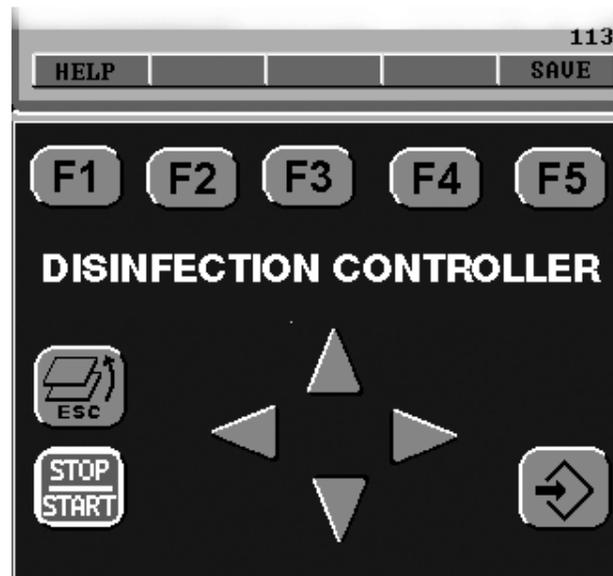
The **START/STOP key** is used to start or stop overall controlling or dosing. In this case, the permanent display and the main center menu option show "Dosing ON" or "Dosing OFF".
