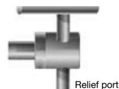
Backpressure valve on tee for pressure relief
