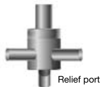
In-line pressure relief valve (3 port)
