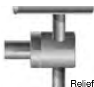
Backpressure valve on tee for pressure relief
