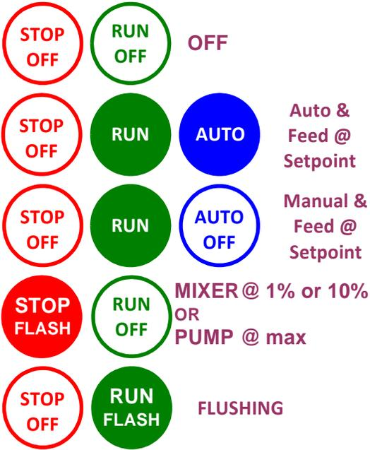
The enclosure door lights complement the LCD state display messages & understandably can be seen from a greater distance than the LCD display.
