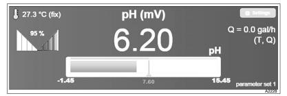
Fig. 2: Main display of a channel
