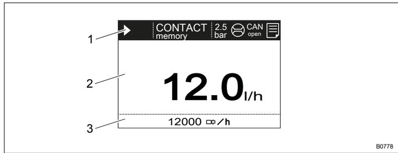
Fig. 5: Construction of the continuous display
