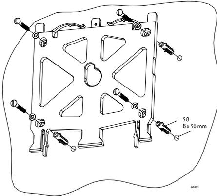
*Fig. 8: Fitting the wall bracket*
