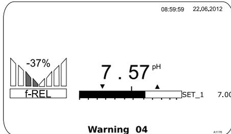
Fig. 3: This is the appearance of the continuous display when used with one measuring channel (e.g. pH)
