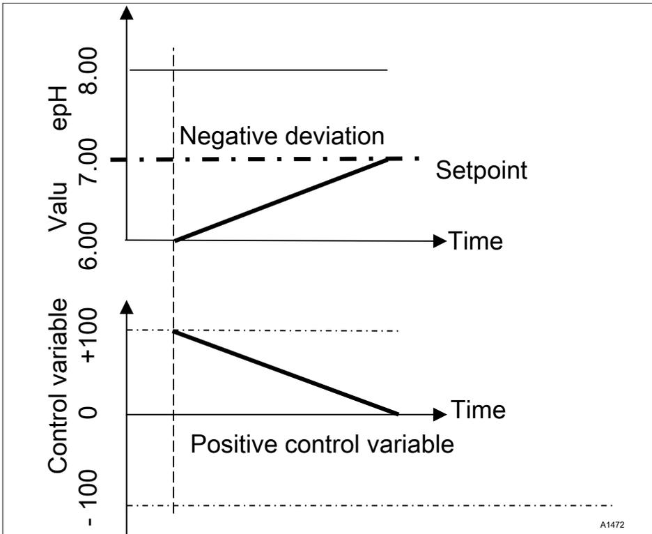
Fig. 77: Control type 1-way PID, direction pH increase value
