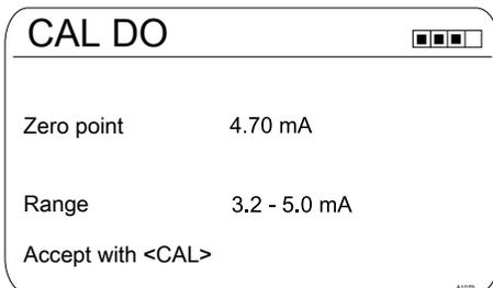
*Fig. 66: Zero point calibration for the measured variable DO*
