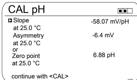
Fig. 40: Selection of the settable parameters
