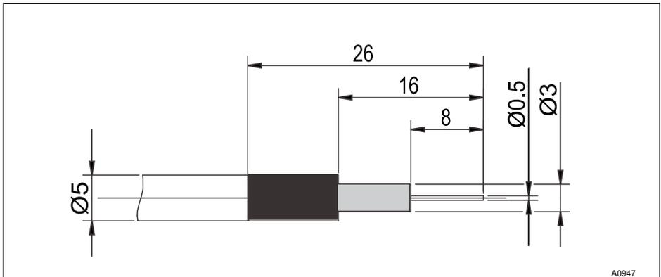
Fig. 24: Coaxial cable assembly
