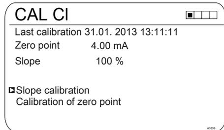
Fig. 28: Display [Calibrate] in the example [Cl] (chlorine)
