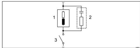
*Fig. 22: RC protective circuit for the relay contacts*
