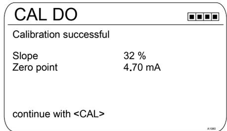
*Fig. 67: Zero point calibration for the measured variable DO*
