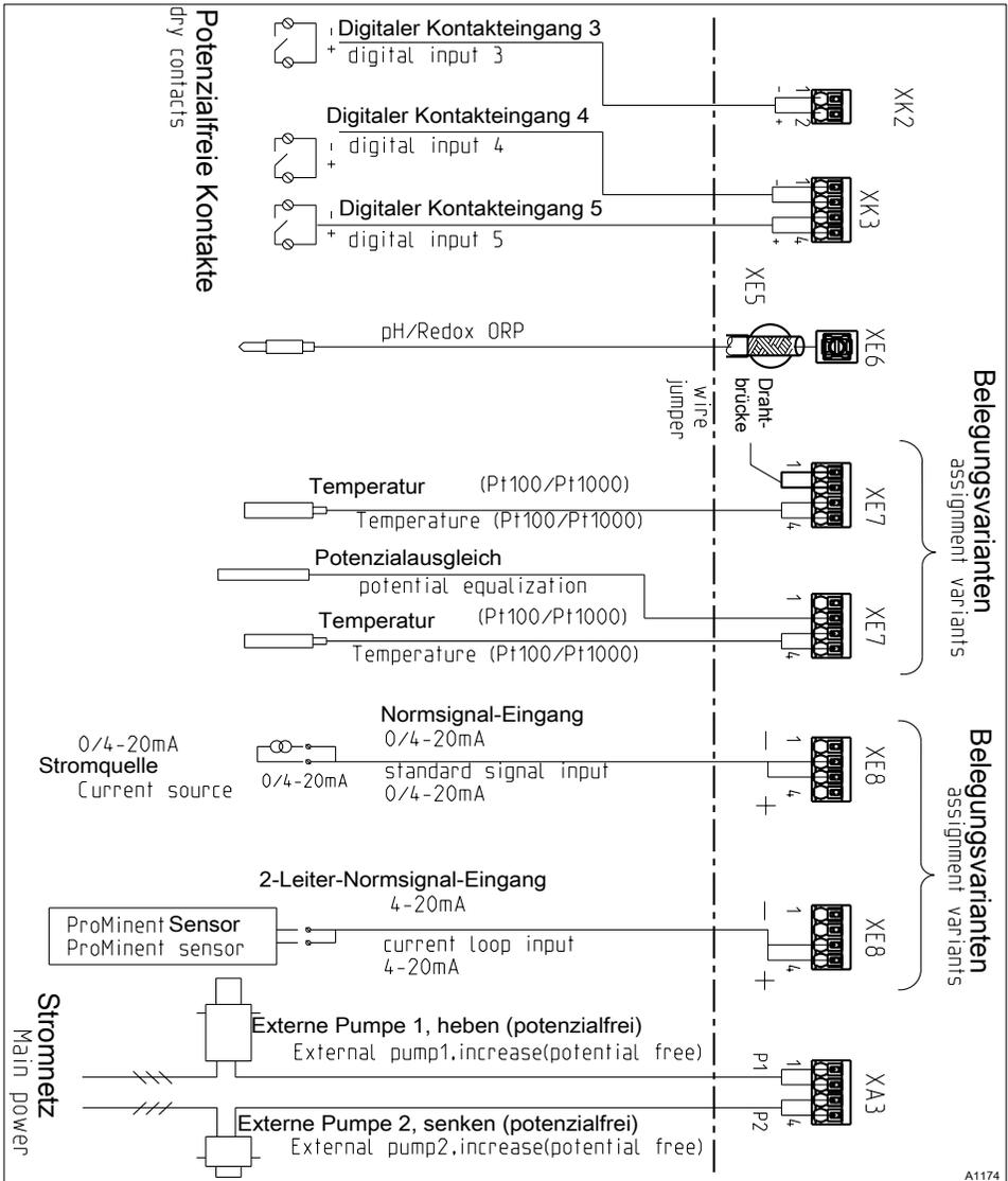
Fig. 17: Terminal diagram with assignment variants
