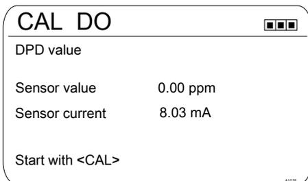
*Fig. 69: DO value calibration for the measured variable DO*
