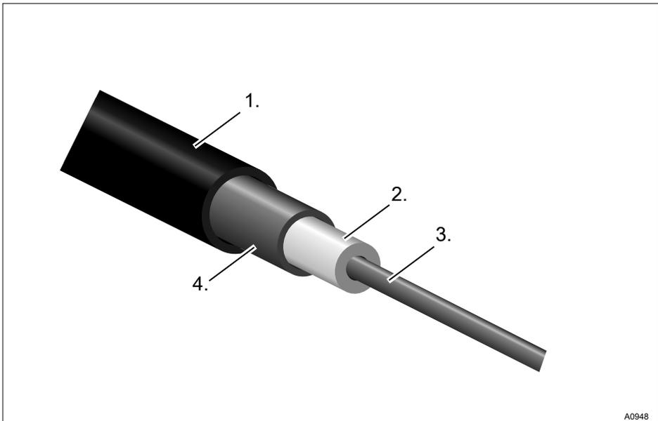
Fig. 23: Coaxial cable cutaway view:
