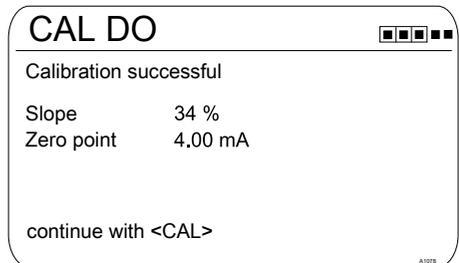
*Fig. 71: DO value calibration for the measured variable DO*
