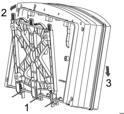
*Fig. 9: Fitting the wall bracket*
