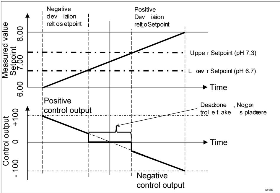
Fig. 75: Control type two-way PID, with dead zone
