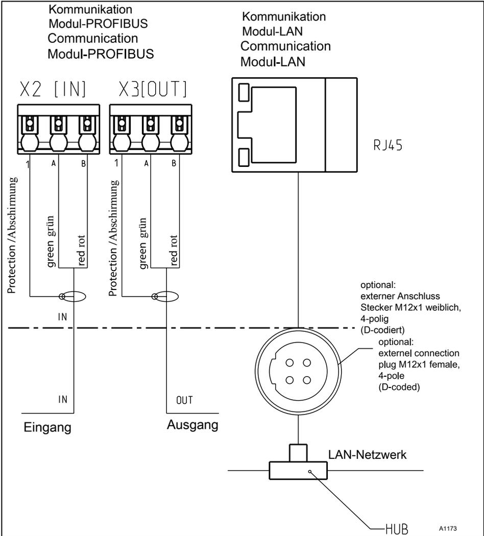
Fig. 19: Terminal diagram DAC "communication module"
