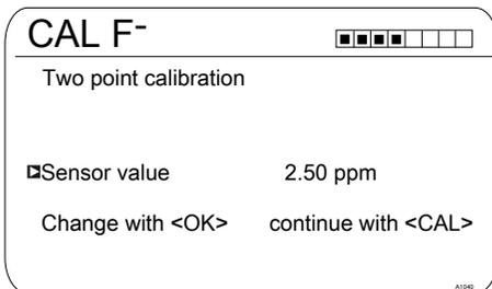
Fig. 52: Fluoride sensor calibration (CAL)
