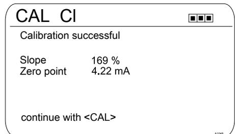
Fig. 61: Calibration of zero point
