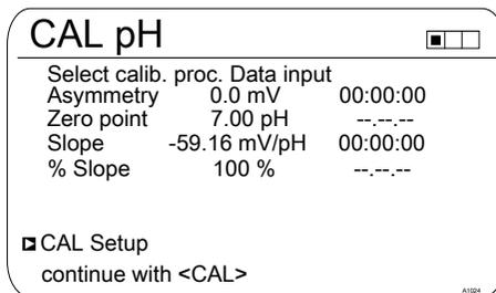
Fig. 39: pH sensor calibration (CAL)
