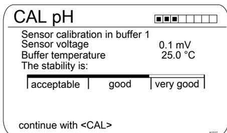
Fig. 34: Display of the attained sensor stability
