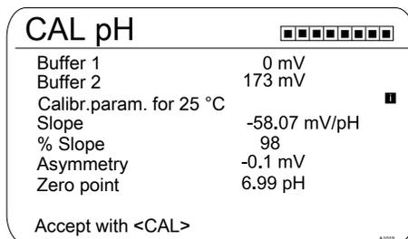
Fig. 36: Display of the calibration result
