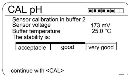
Fig. 35: Display of the attained sensor stability
