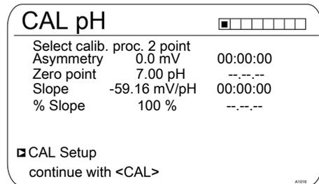
Fig. 33: pH sensor calibration (CAL)
