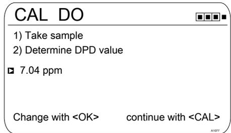
*Fig. 70: DO value calibration for the measured variable DO*
