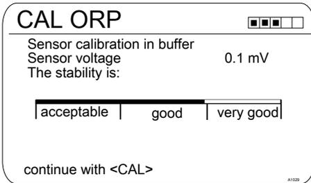
Fig. 44: Display of the attained sensor stability
