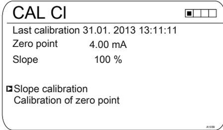
Fig. 56: Calibration menu [Chlorine]
