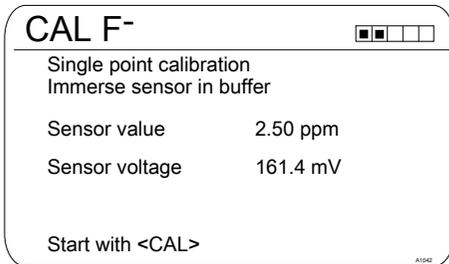
Fig. 54: Fluoride sensor calibration (CAL)
