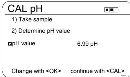
Fig. 38: Work instruction for determining the pH value using the [Sample] method
