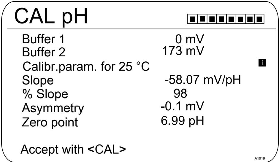
Fig. 29: Display of the calibration result
