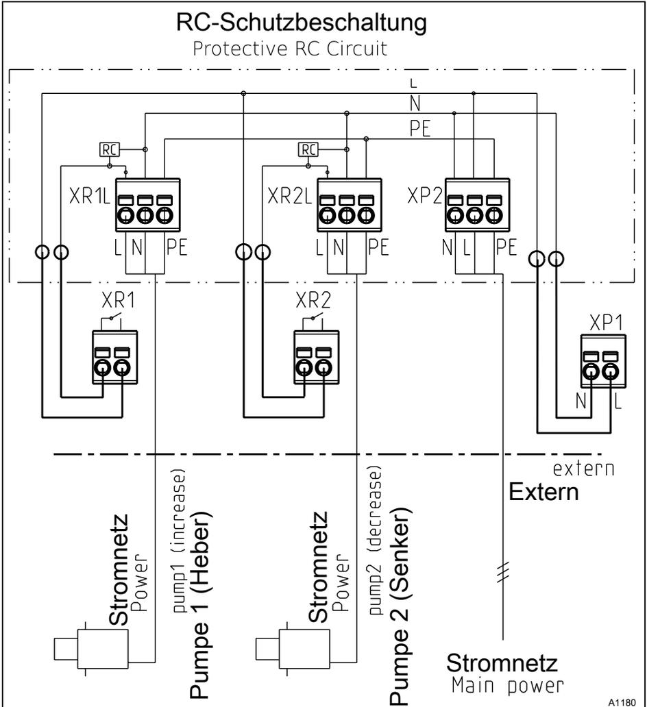
Fig. 18: Terminal diagram with protective RC circuit (option)
