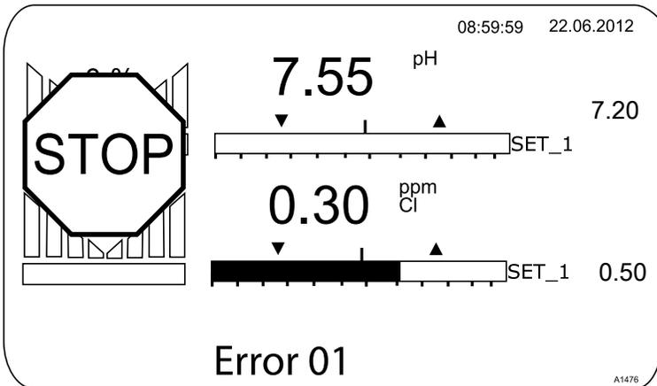
Fig. 6: Alarm message, controller stops control
