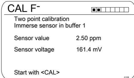
Fig. 51: Fluoride sensor calibration (CAL)
