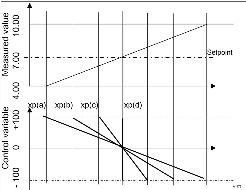
Fig. 78: The smaller the xp value, the more "forcefully" the control reacts.
