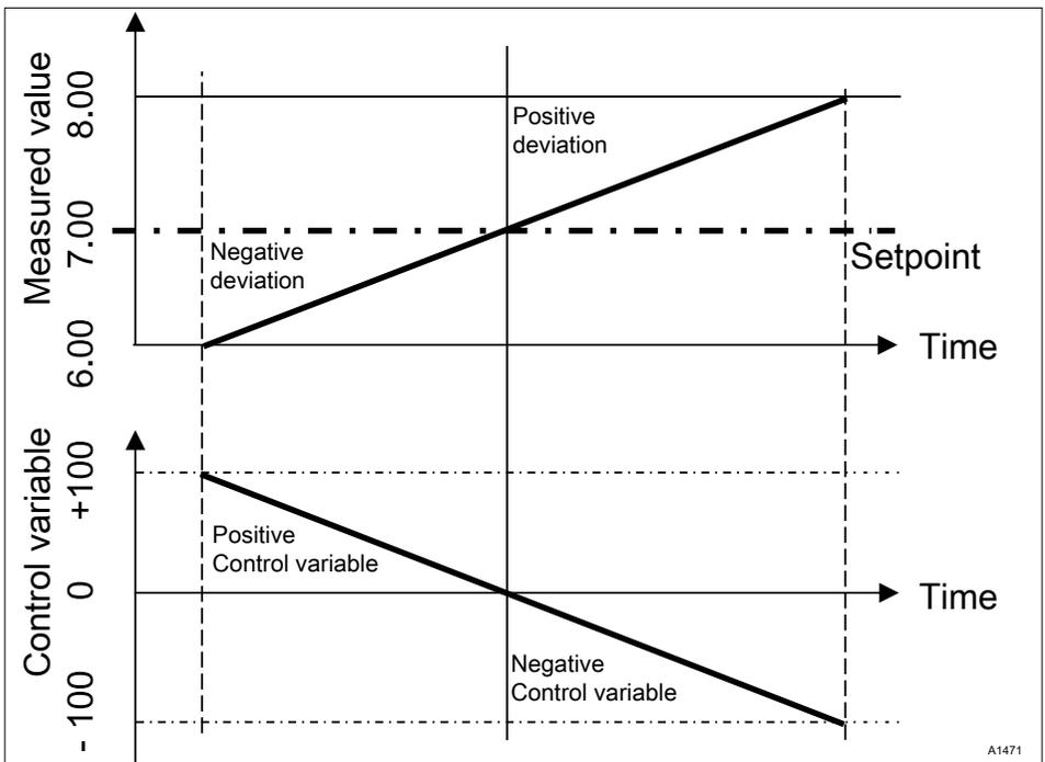
Fig. 74: Control type two-way PID. Control characteristic without dead zone
