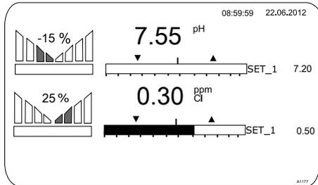
Fig. 4: This is the appearance of the continuous display when used with two measuring channels (e.g. pH/chlorine)
