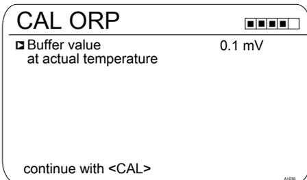
Fig. 45: Adjusting the buffer value
