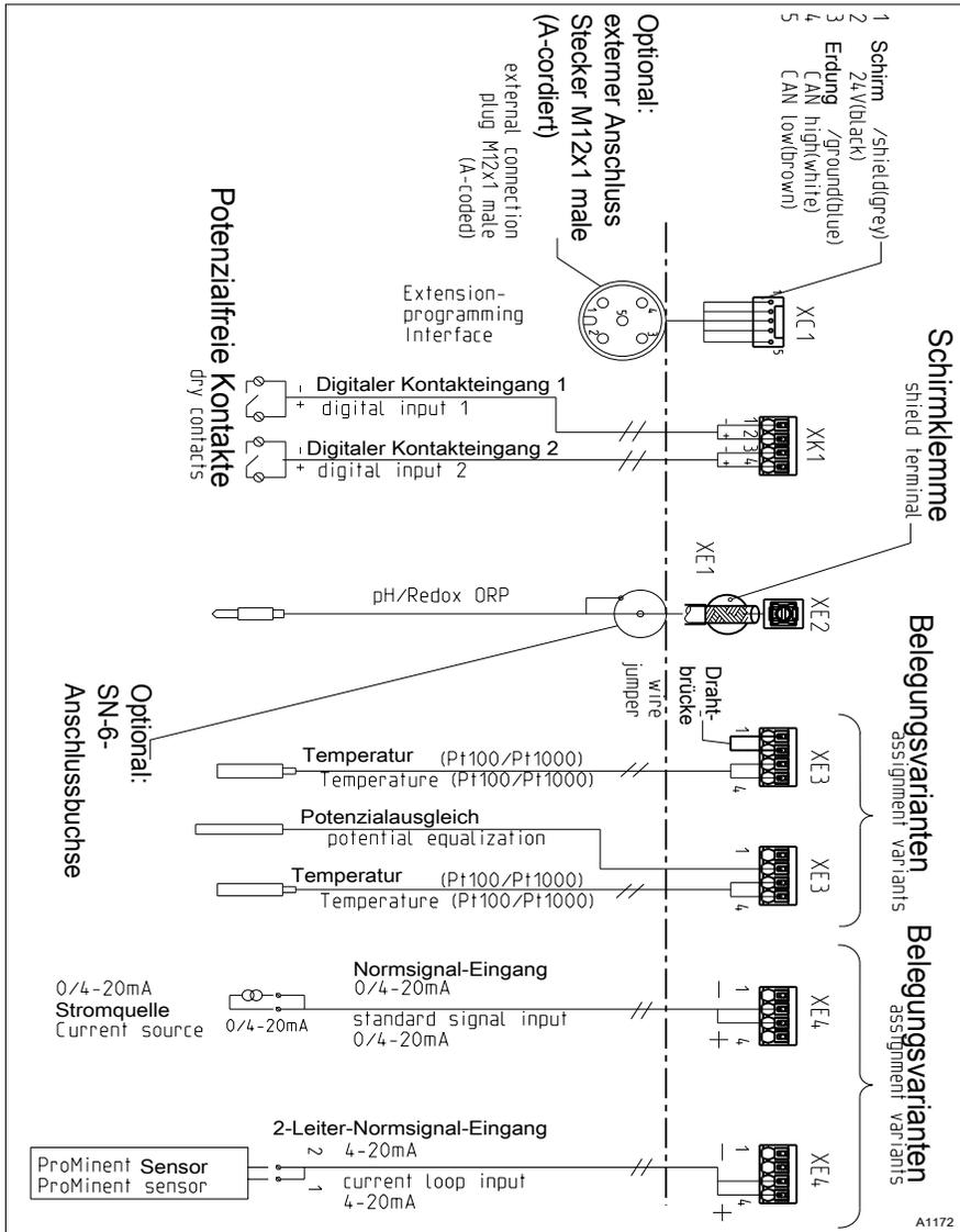
Fig. 15: Terminal diagram with assignment variants
