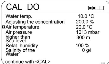
*Fig. 68: DO value calibration for the measured variable DO*
