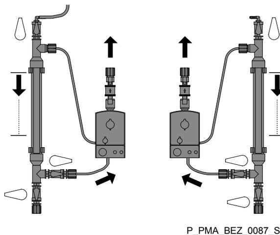
Fig. 14: Stopcock positions during calibration, shown here for CDVc
