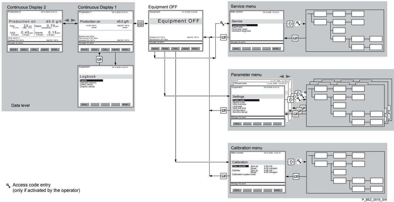
Fig. 12: Operating menu, schematic
