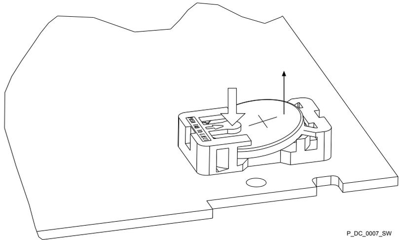
*Fig. 23: Removing the battery*
