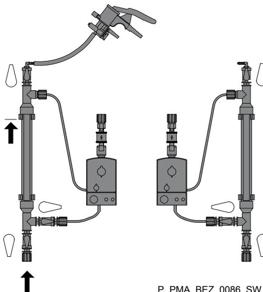
Fig. 13: Stopcock positions during filling of the calibration devices, shown here for CDVc
