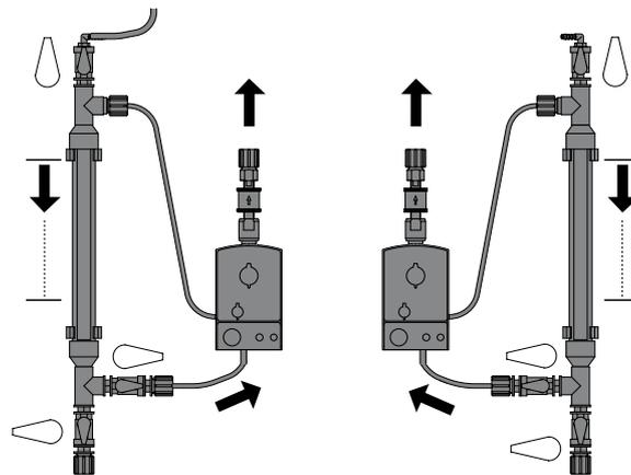
Fig. 18: Stopcock positions during calibration, shown here for CDVc
