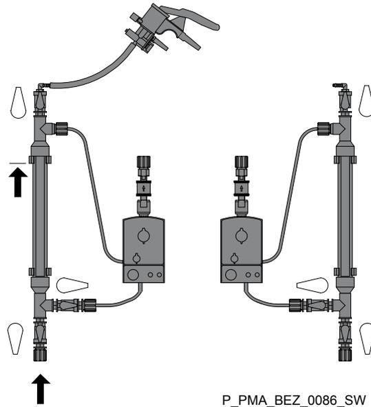
Fig. 17: Stopcock positions during filling of the calibration devices, shown here for CDVc
