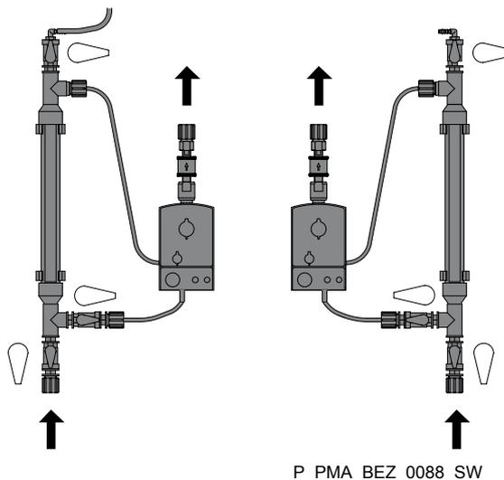
Fig. 15: Stopcock positions in operation, shown here for CDVc
