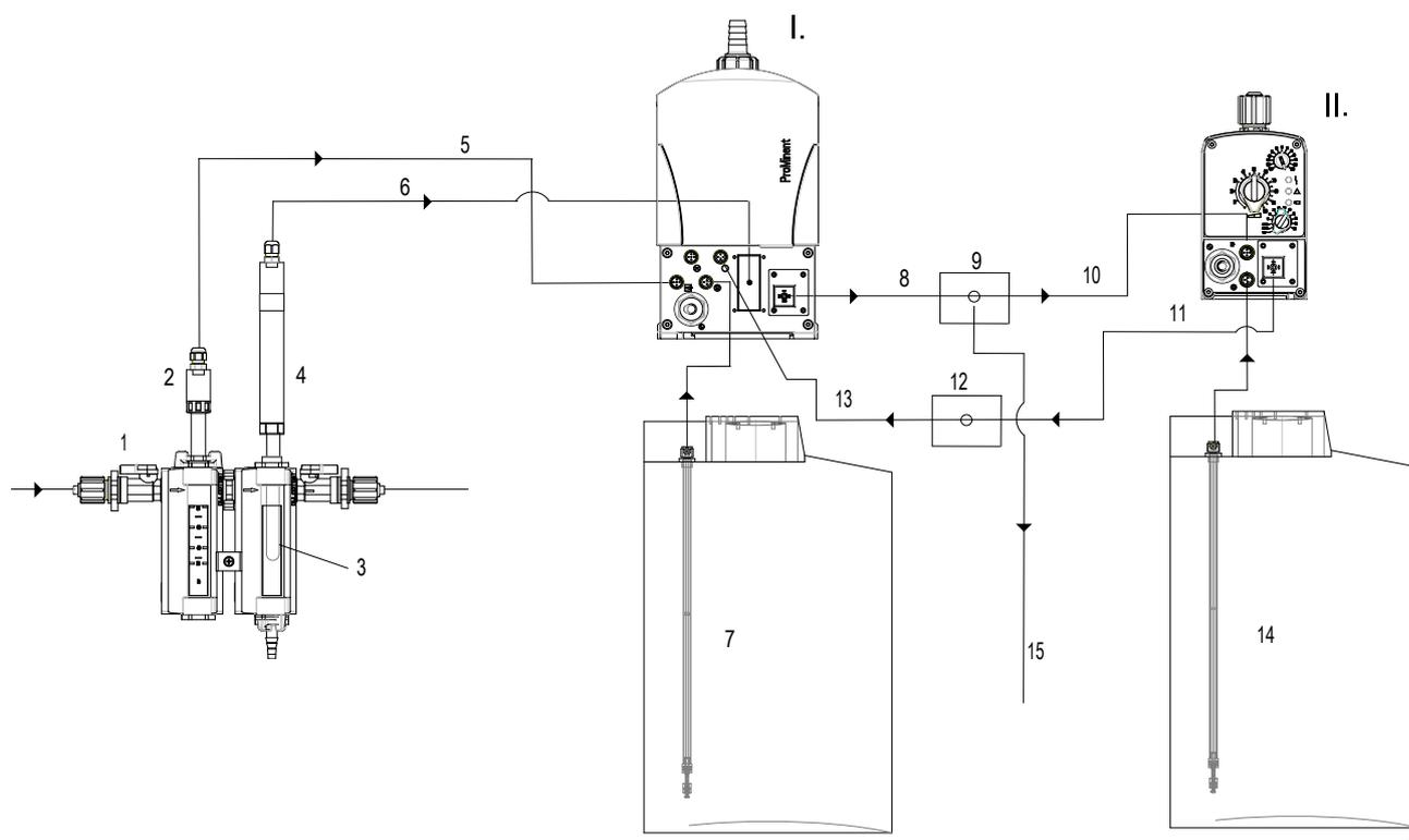
Fig. 2: Application example of pH or redox system for two-sided control
