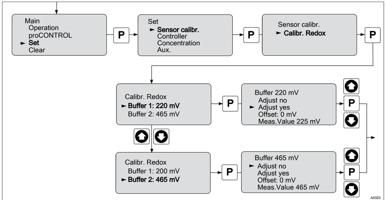
Fig. 27: Calibrating the sensor for Redox
