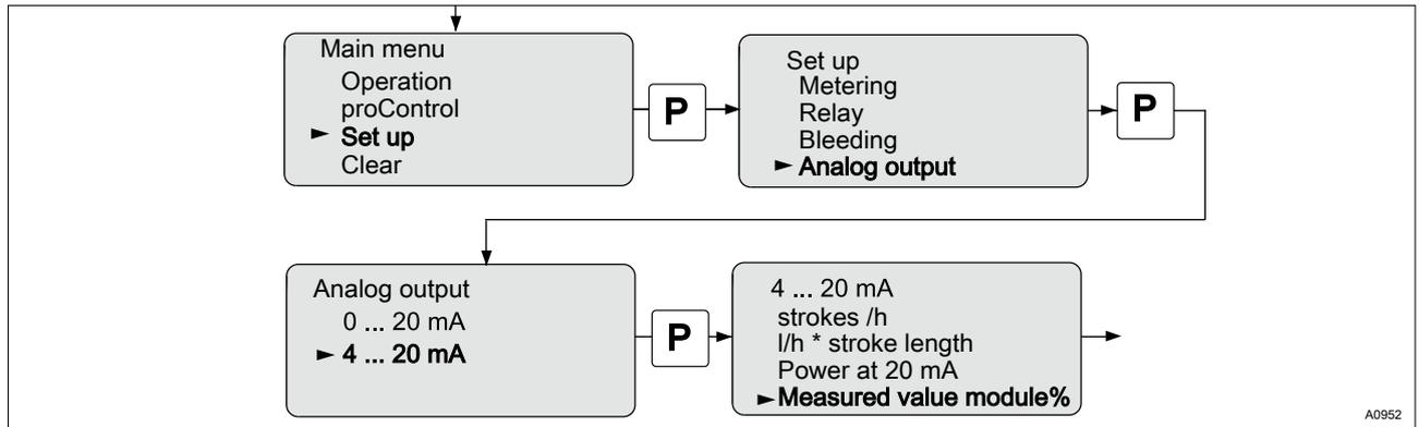
Fig. 24: Current output activation menu
