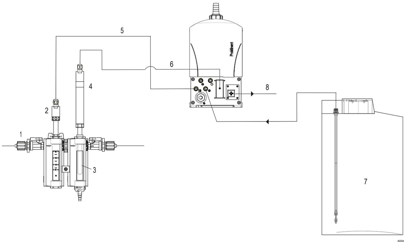
Fig. 1: Application example of pH or redox system for one-sided control
