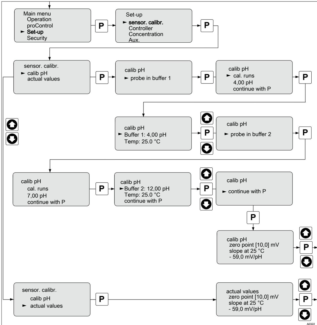
Fig. 26: Sensor pH calibration
