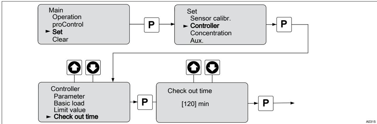
Fig. 19: Checkout time adjustment
