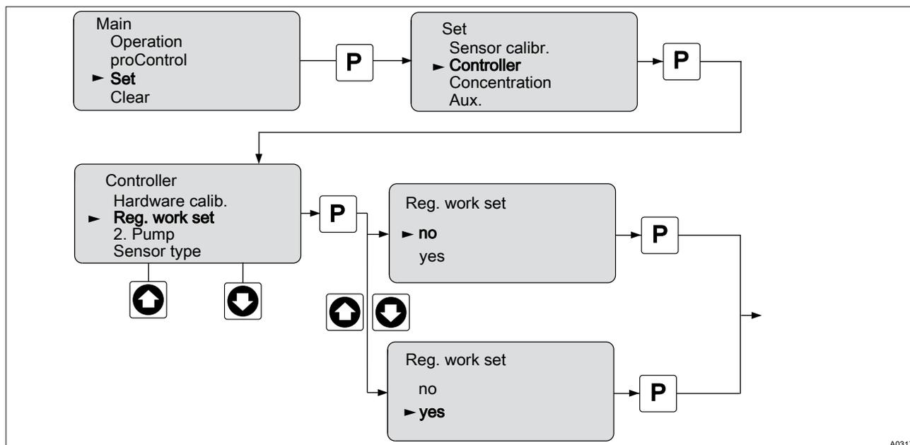
Fig. 21: Factory settings of the control module delta®
