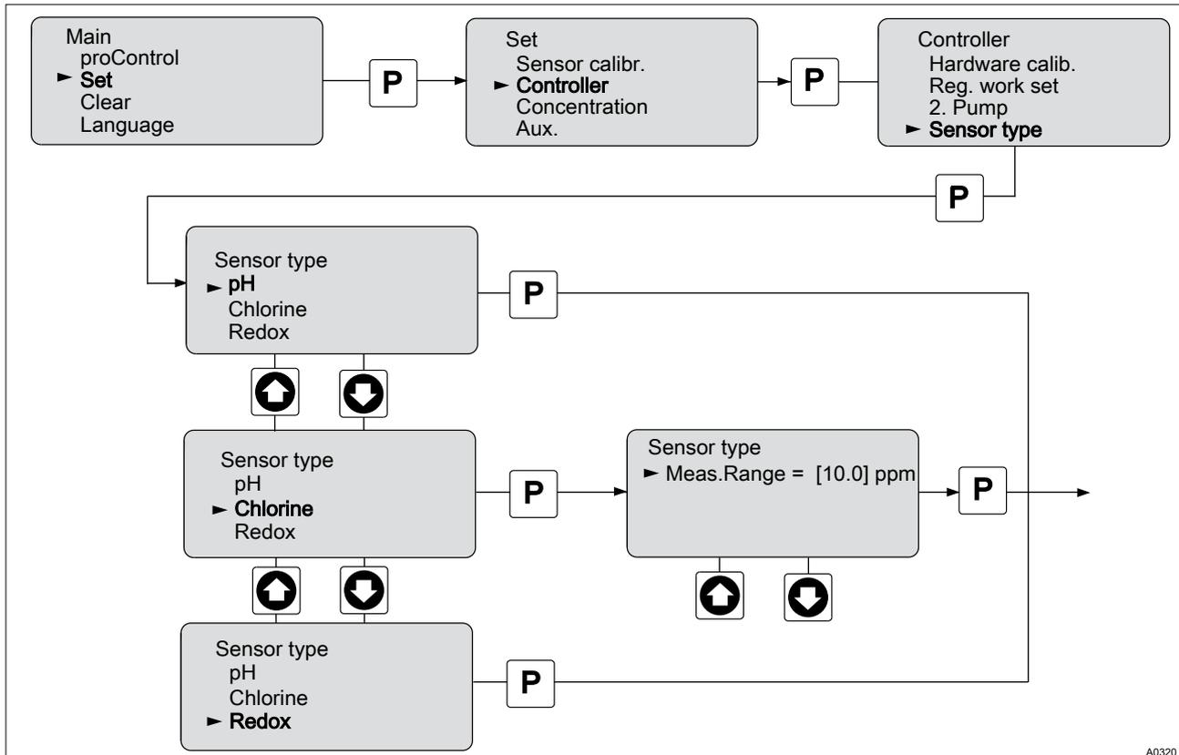
Fig. 15: Selection of the Measured Variable and Measuring Range
