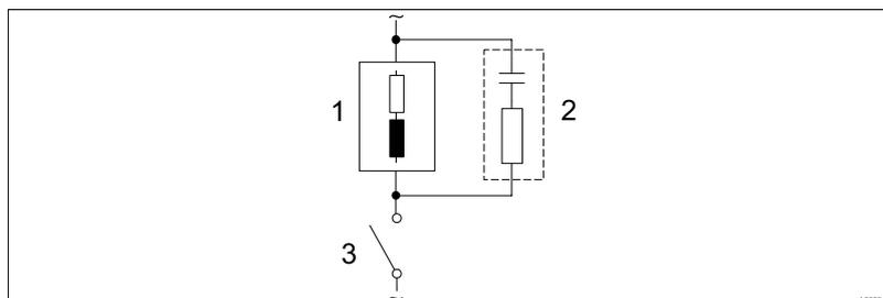
Fig. 10: RC protective circuit for the relay contacts
