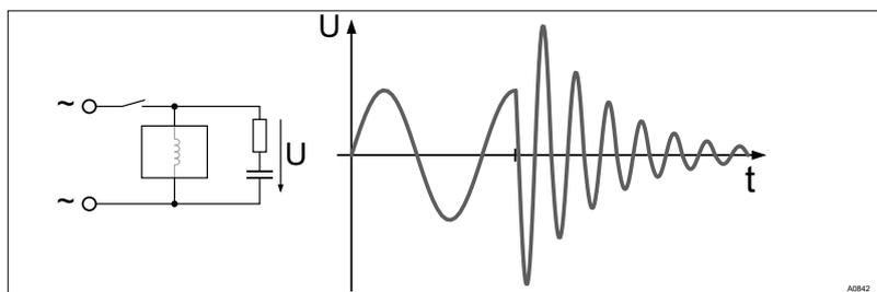
Fig. 9: Switching-off process shown on the oscillogram.
