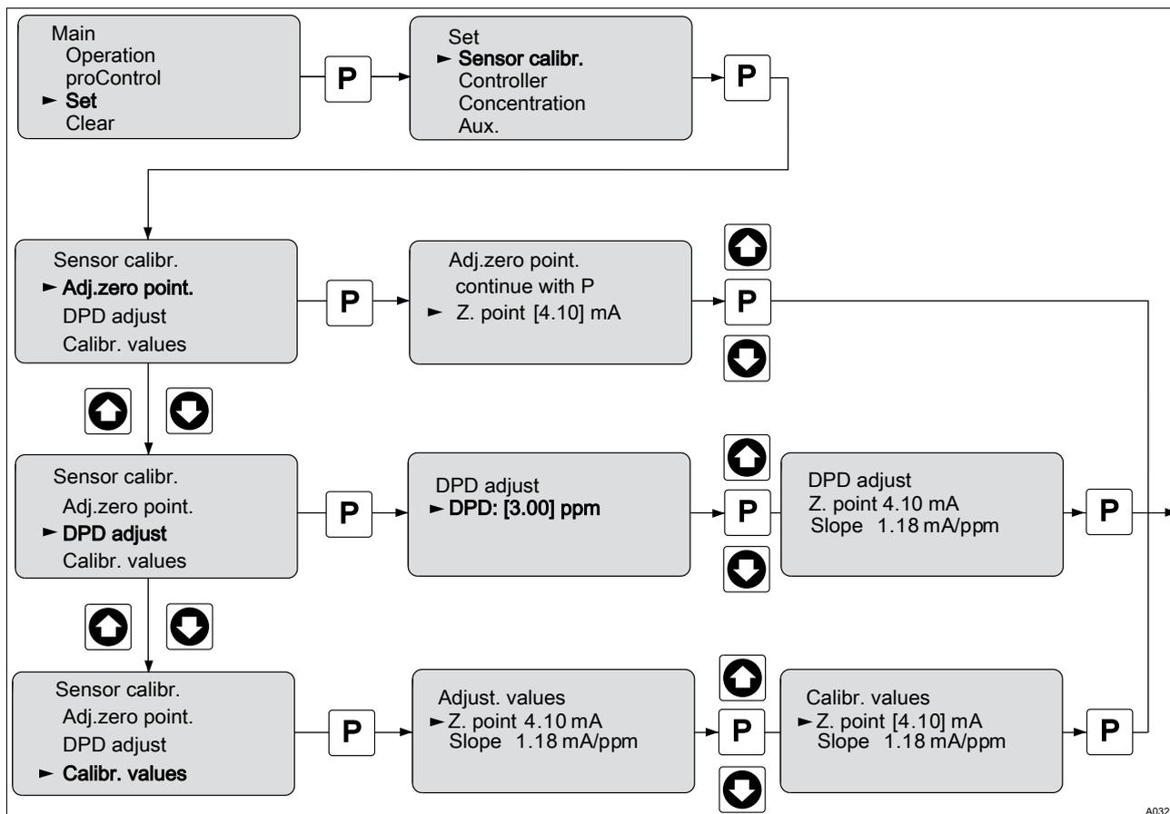
Fig. 25: Calibrating the sensor for chlorine
