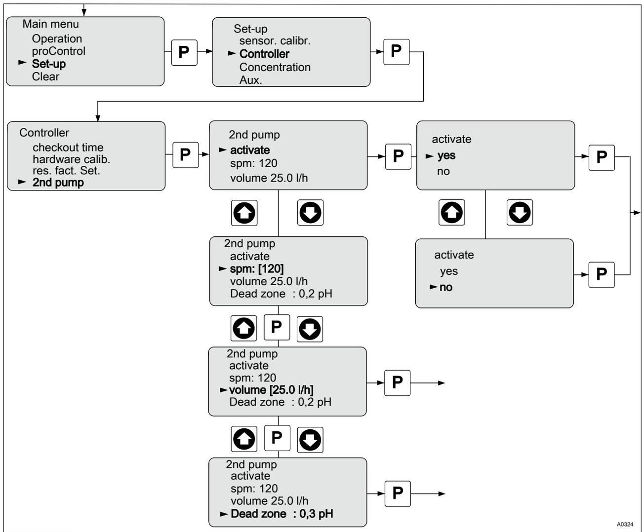
Fig. 22: Setting up "Two pump operation"
