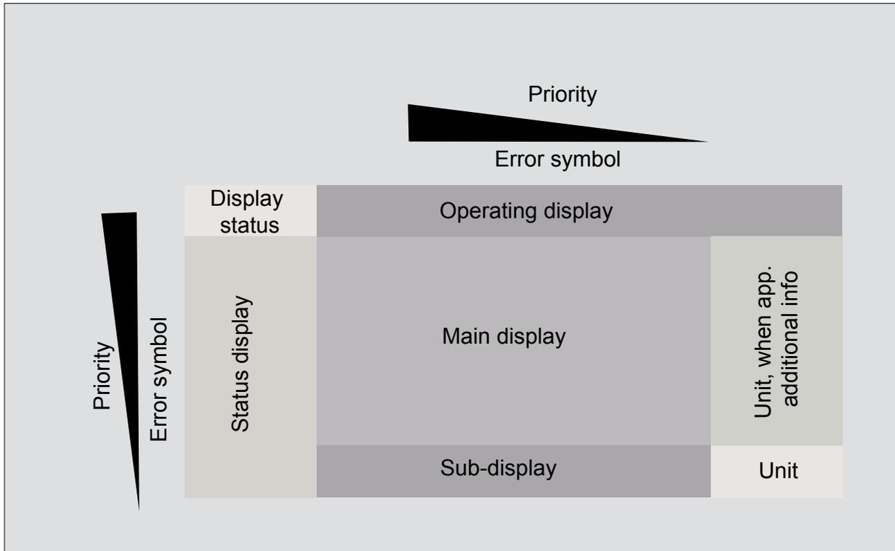
Fig. 28: Overview of the operating indicator of the delta® solenoid metering pump
