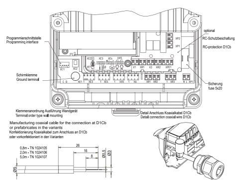
Fig. 9: Preparation of coaxial cable
