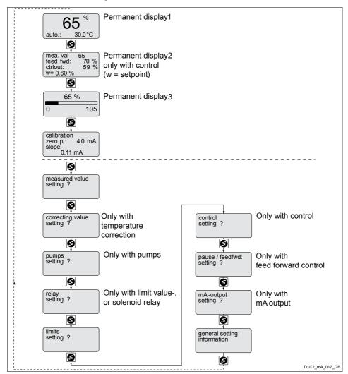
Fig. 52: Complete operating menu / Shown with measured variable % and the measuring range 0%....100%
