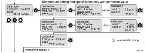
Fig. 46: Calibrating the fluoride sensor
