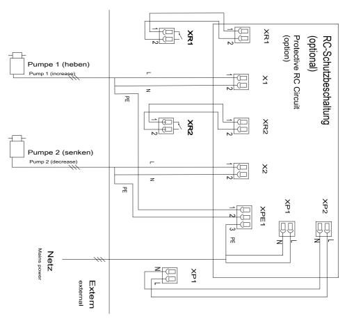
Fig. 13: Protective RC circuit terminal diagram
