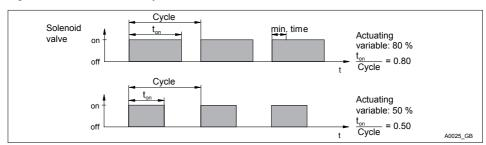
Fig. 62: Solenoid valves
