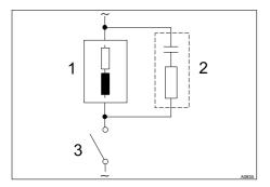
Fig. 22: RC protective circuit for the relay contacts
