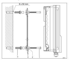
Fig. 3: Fixing material for wall mounting
