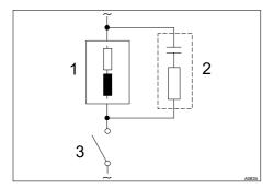
Fig. 15: RC protective circuit for the relay contacts
