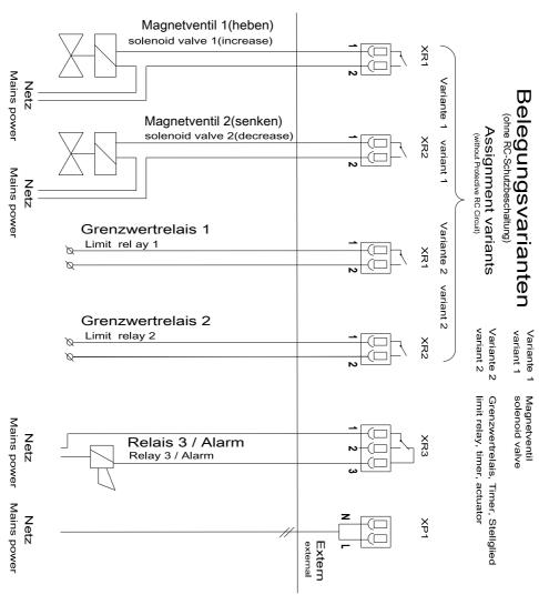
Fig. 11: Terminal diagram with assignment options 1
