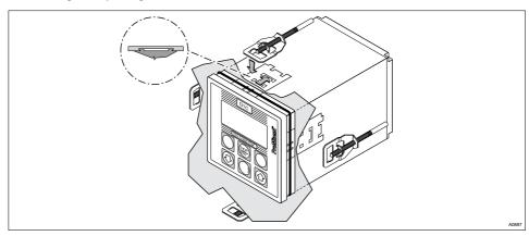
Fig. 17: Screw the studs forward
