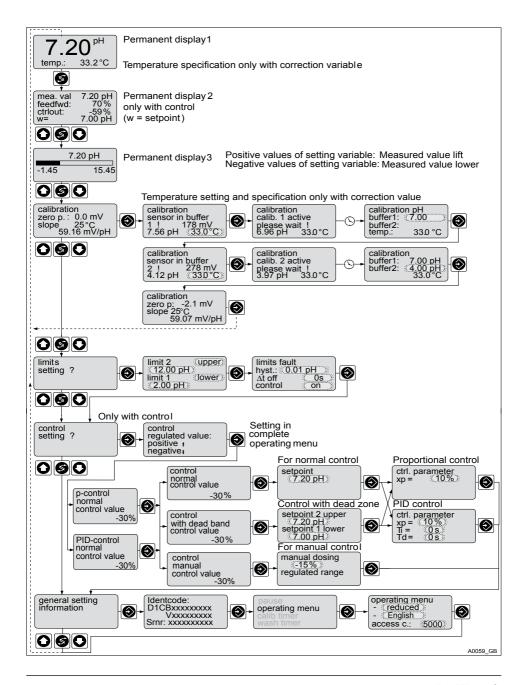
Fig. 42: Reduced pH / redox / fluoride operating menu (shown with the example of pH)
