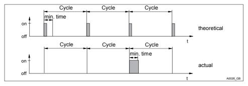
Fig. 63: Theoretical switching time < min. time
