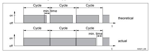
Fig. 64: Theoretical switching time > (cycle - min. time) and calculated switching time < cycle
