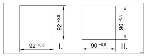
Fig. 16: Mounting - control panel installation DULCOMETER® D1Cc
