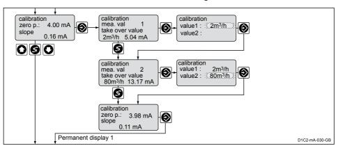
Fig. 54: Two point calibration menu / shown with flow as the measured variable and the measuring range  $0...100 \text{ m}^3/\text{h}$
