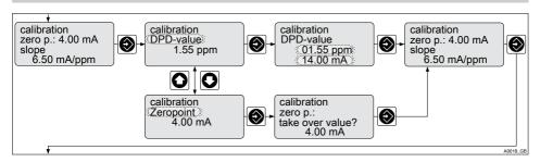
Fig. 38: Calibration of All Amperometric Measured Variables
