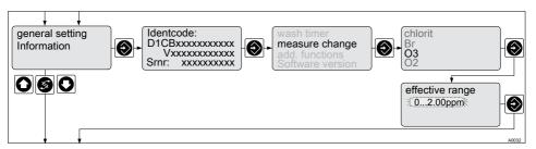
Fig. 24: Selection of measured variable and measuring range
