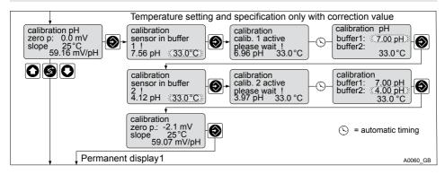
Fig. 44: Calibration of pH sensors
