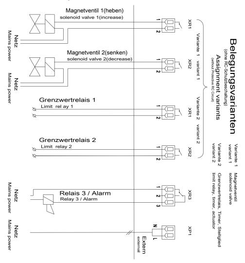
Fig. 19: Terminal diagram with assignment options 1
