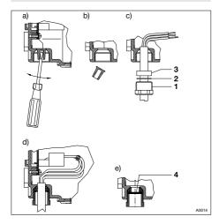
Fig. 7: Punching out the threaded holes
