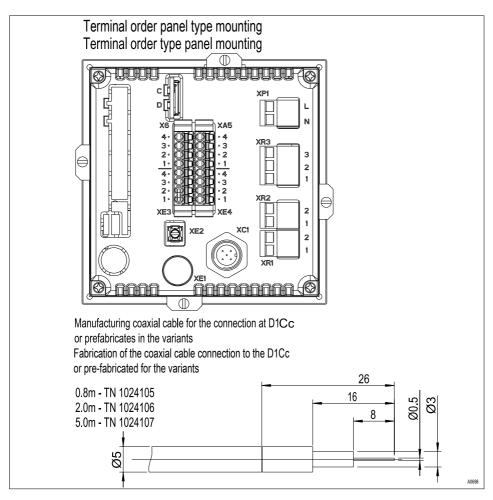
Fig. 18: Preparation of coaxial cable
