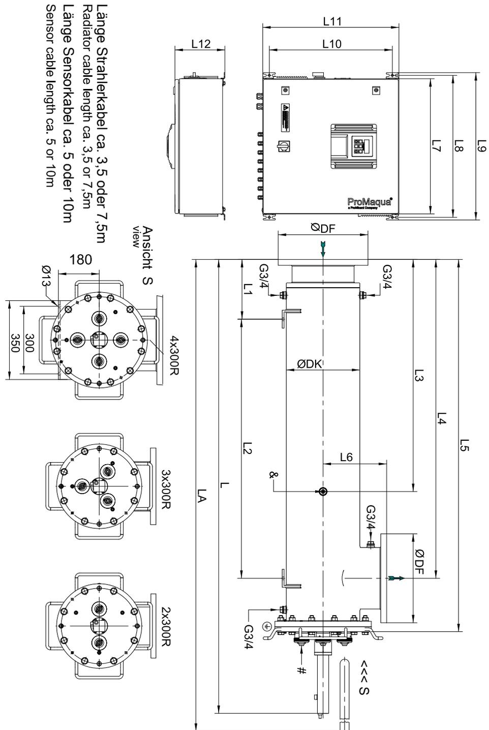
Fig. 52: Data sheet Dulcodes R with automatic wiper
