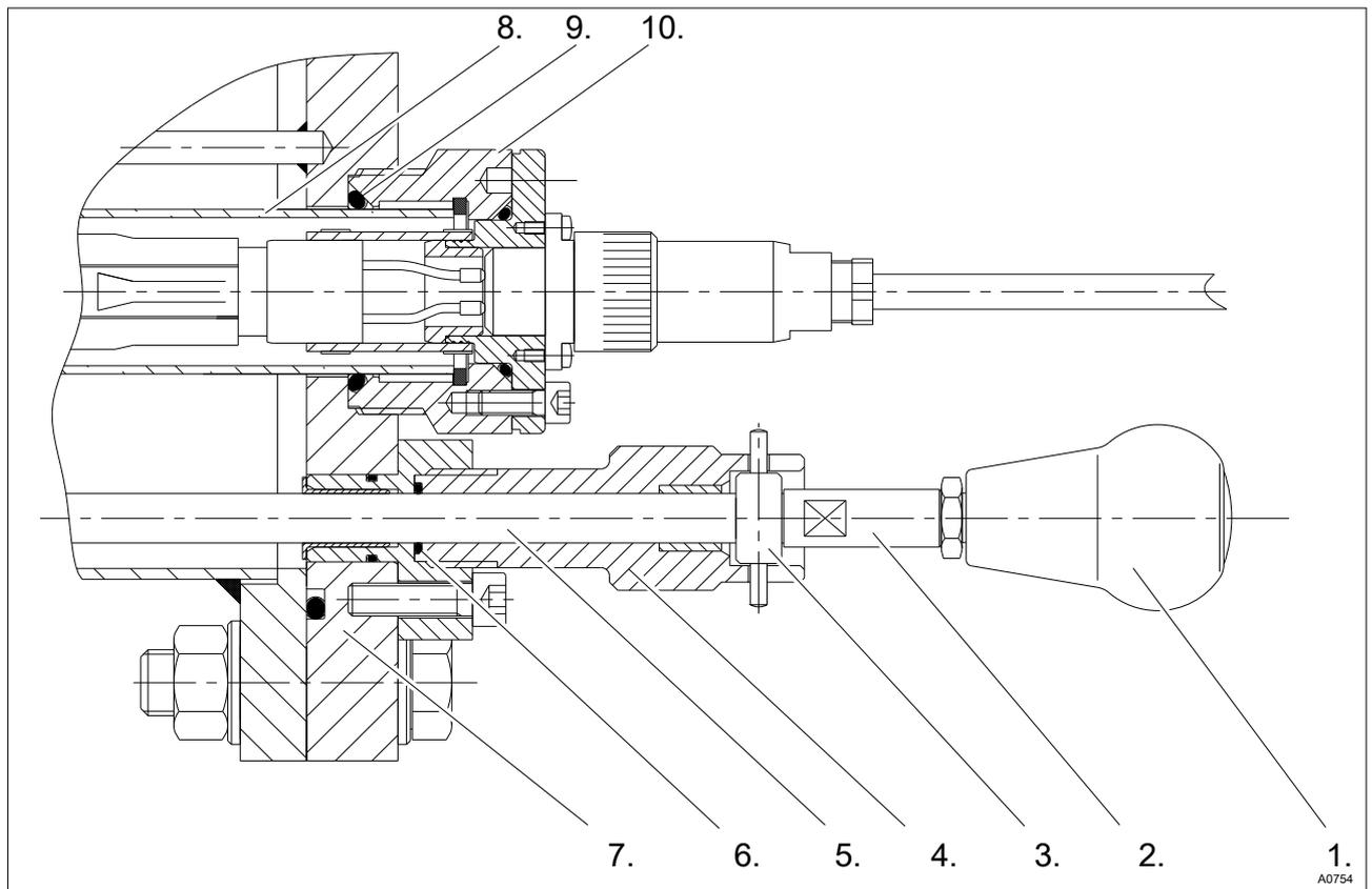
Fig. 30: Components of the manual wiper on the chamber cover and parts of the UV lamp
