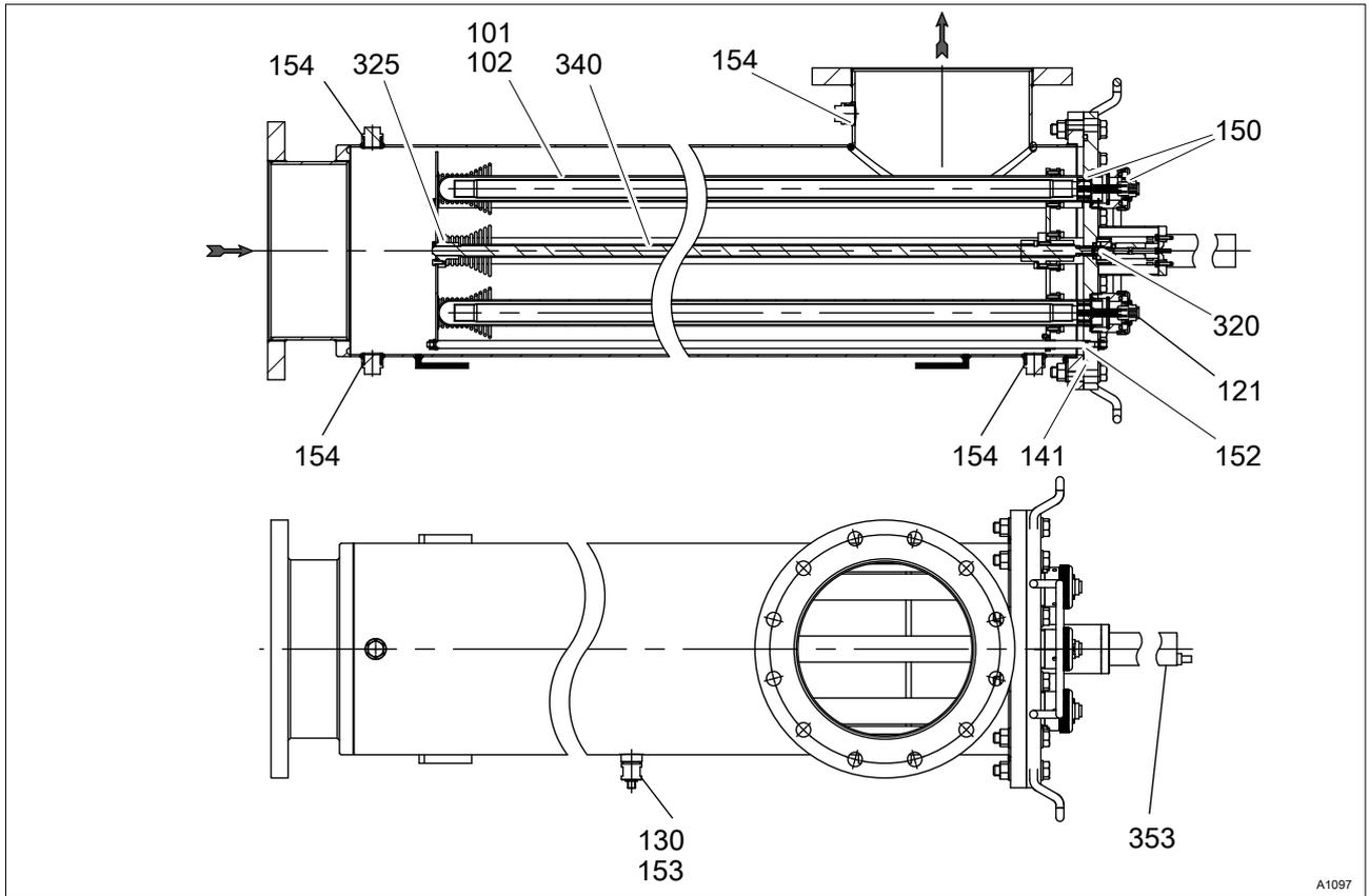
Fig. 55: Spare parts drawing Dulcodes R
