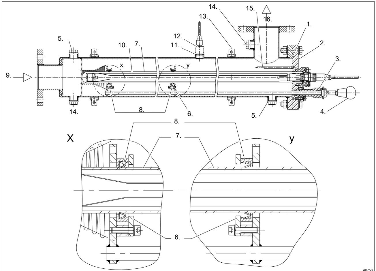
Fig. 28: Construction of the radiation chamber with detail X and Y for the example of a Dulcodes 1x300 R with manual wiper
