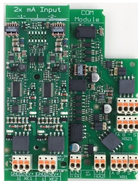
Driver card installed on Com module
