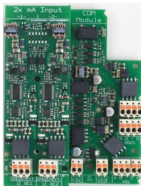
Driver card installed on Com module
