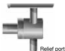
Backpressure valve on tee for pressure relief
