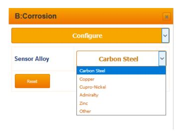
A corrosion rate sensor should never be calibrated. Open the Configuration menu and select the Alloy you are using. Press Submit
