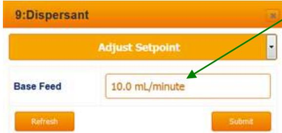
Relay 1-5 controlled base feeds are the same as Pulse 6-9 outputs configured **Mode = ON/OFF output** with **Set Feed Mode = Percent Time & Submit**
