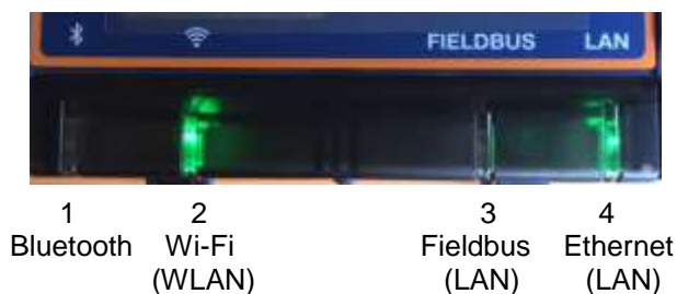
Figure 3 Communication Status LEDs (Bluetooth and Fieldbus are not currently available. Jan 2017)
