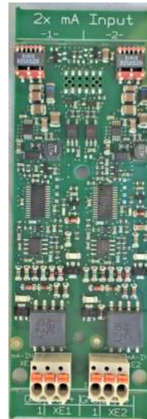
Figure 54 Dual 4-20mA Input driver
