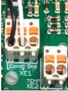
Figure 41 Two Wire Boiler Probe on XE1
