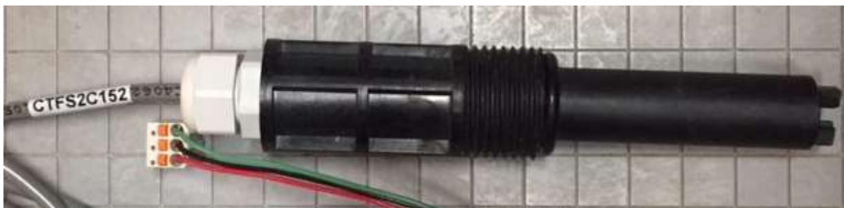
Figure 38 CTFS sensor (Conductivity/Temperature/Flowswitch/Serial)
