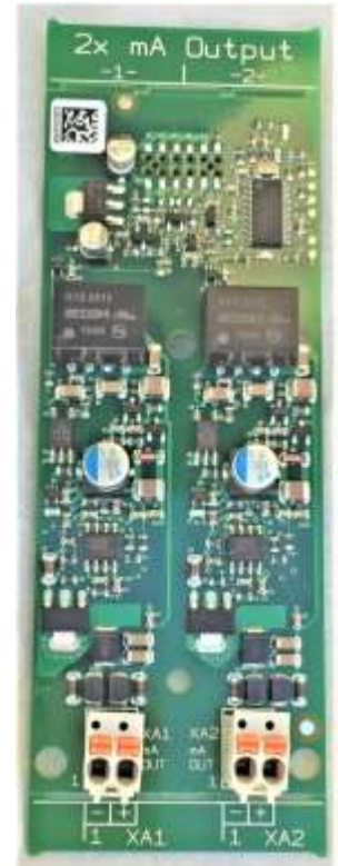
Figure 58 Dual 4-20mA Output driver
