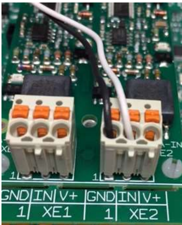
Figure 57 Two wire remotely powered Analog input
