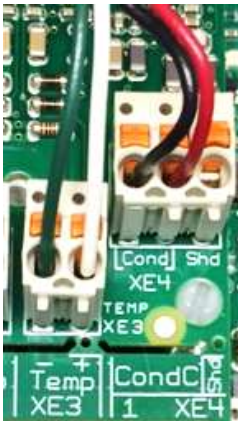
Figure 43 Four Wire Condensate Probe On XE2
