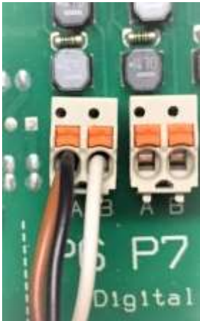
Figure 30 Universal Control Cable on Output Relay P6
