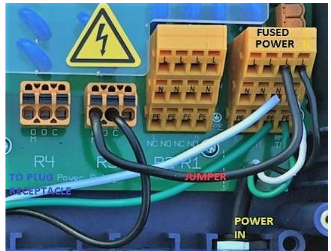
Figure 25 Wiring R3 using on-board fused power
