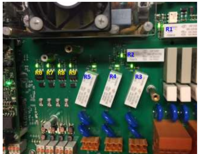
Figure 12 Internal Relay Indicator LEDs
