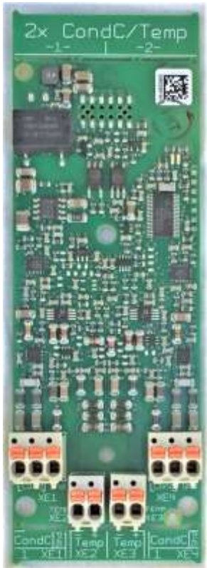
Figure 40 Dual Conductivity Driver
