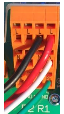
Figure 24 R1 MOV Wiring example
