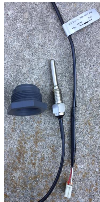
Figure 69 PT1000 Black cable 2-wire temperature sensor 1080101, with DGMA adapter 1051504. Assembly PN 1002856
