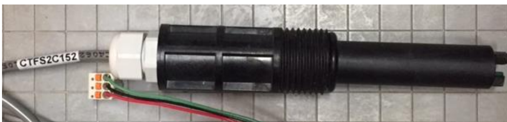
Figure 38 CTFS sensor (Conductivity/Temperature/Flowswitch/Serial)
