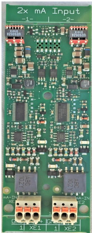
Figure 54 Dual 4-20ma Input driver
