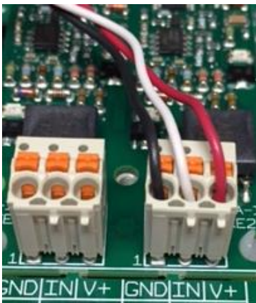
Figure 56 Three wire 4-20mA inputs that utilize V+
