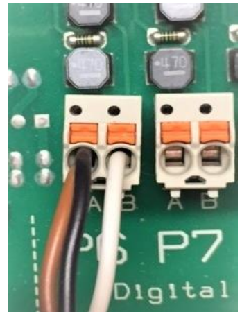
Figure 30 Universal Control Cable on Output Relay P6
