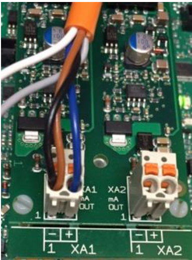
Figure 63 Dual mA Output with ProMinent Universal Control Cable on output 1.
