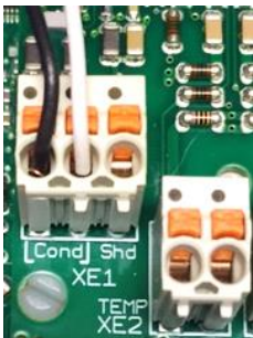
Figure 41 Two Wire Boiler Probe on XE1
