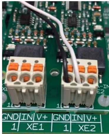
Figure 57 Two wire remotely Powered Analog input
