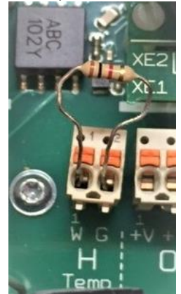
Figure 33 Input H with test resistor
