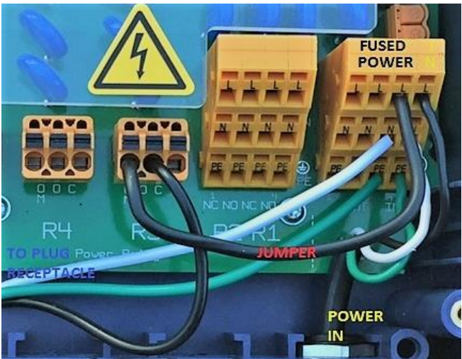
Figure 25 Wiring R3 using on-board fused power
