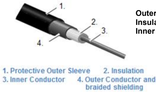
Figure 48 Coaxial Cable Construction
