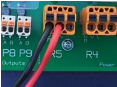
Figure 26 Using external power
