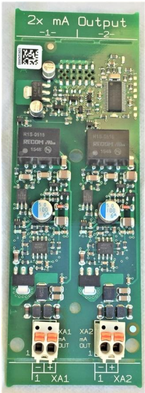
Figure 62 Dual 4-20mA Output driver
