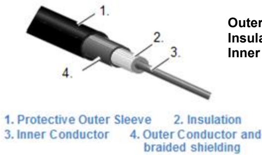
Figure 48 Coaxial Cable Construction
