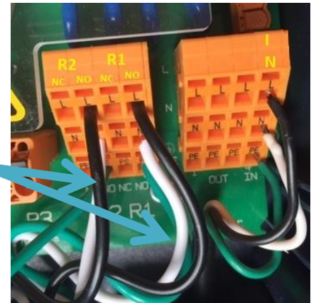
Figure 23 Terminating R1 & R2
