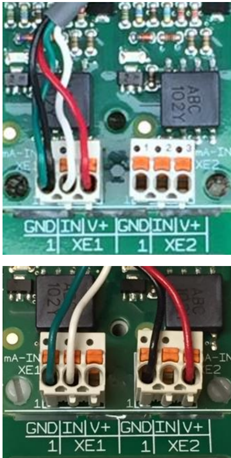
Figure 59 Wiring the Pyxis to a single channel (above) and using the second channel for power (below)
