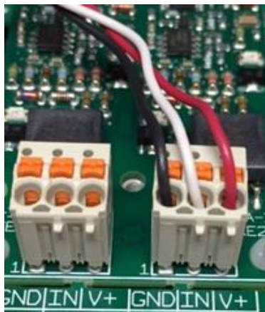
Figure 56 Three wire 4-20mA inputs that utilize V+
