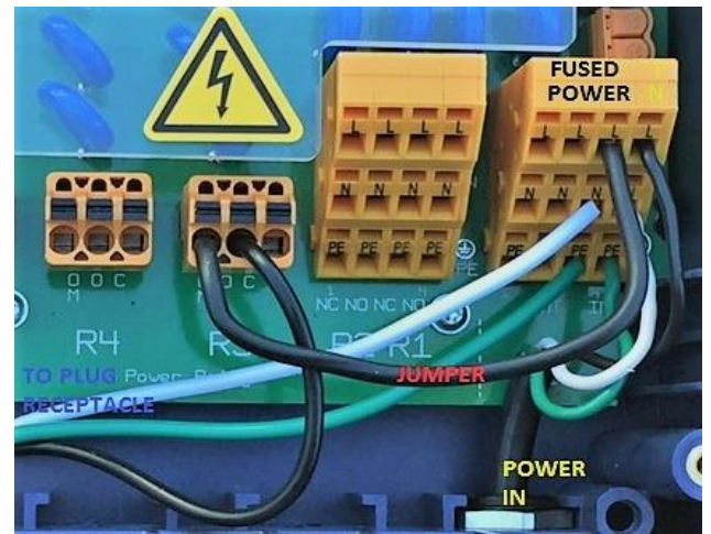
Figure 25 Wiring R3 using on-board fused
