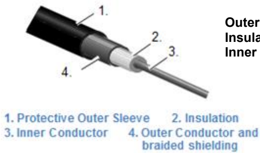
Figure 48 Coaxial Cable Construction
