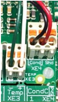
Figure 43 Four Wire Condensate Probe On XE3 (temperature) and XE4 (conductivity).
