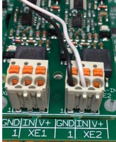
Figure 57 Two wire remotely Powered Analog input
