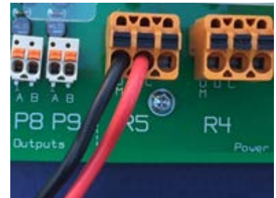
Figure 26 Using external power
