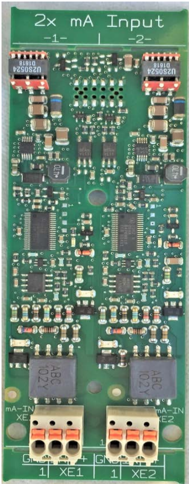
Figure 54 Dual 4-20ma Input driver
