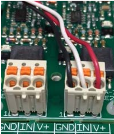
Figure 56 Three wire 4-20mA inputs that utilize V+
