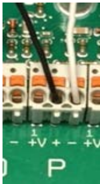
Figure 34 Digital Input wiring
