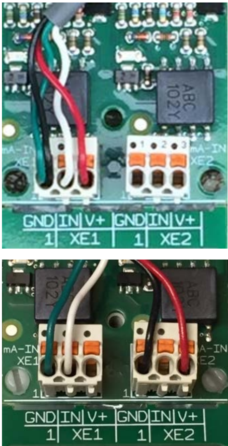
Figure 59 Wiring the Pyxis to a single channel (above) and using the second channel for power (below)
