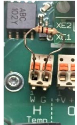
Figure 33 Input H with test resistor
