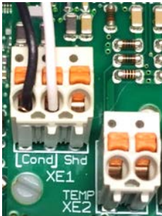
Figure 41 Two Wire Boiler Probe on XE1
