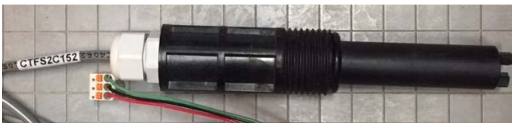
Figure 38 CTFS sensor (Conductivity/Temperature/Flowswitch/Serial)
