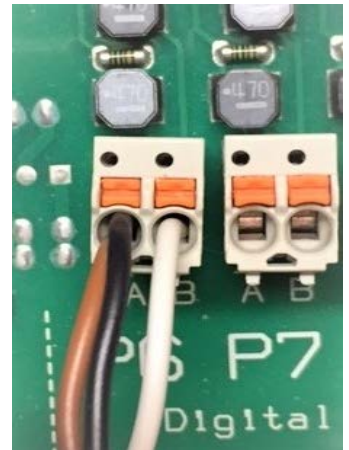
Figure 30 Universal Control Cable on Output Relay P6
