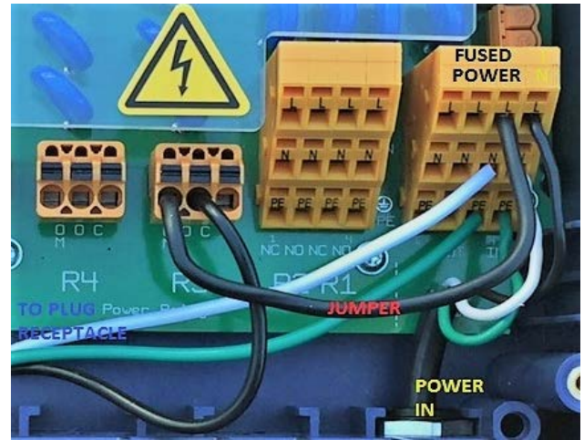
Figure 25 Wiring R3 using on-board fused
