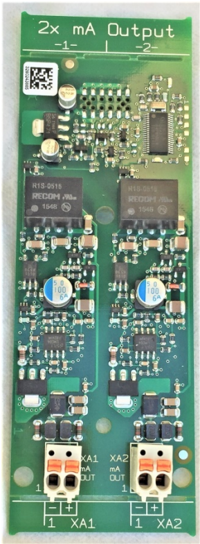
Figure 62 Dual 4-20mA Output driver
