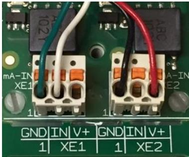
Power can also be provided from the second input. In both ways, the red is on the V+ and black is on the GND terminals.
