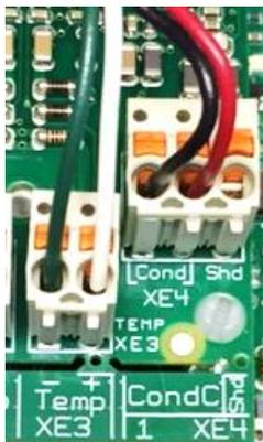
Four Wire Condensate Probe On XE3 (temperature) and XE4 (conductivity).
