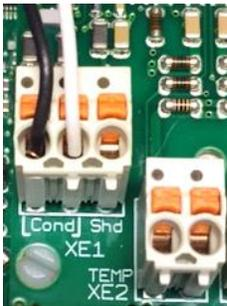
Two Wire Boiler Probe on XE1
