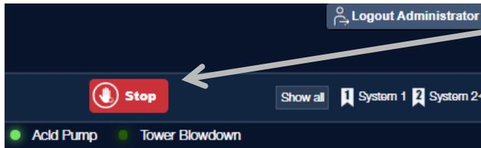
Stop/Start the controller program and disable/enable all outputs. (4-20mA output goes to 4mA)
