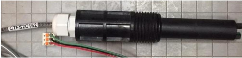
CTFS sensor (Conductivity/Temperature/Flowswitch/Serial)
