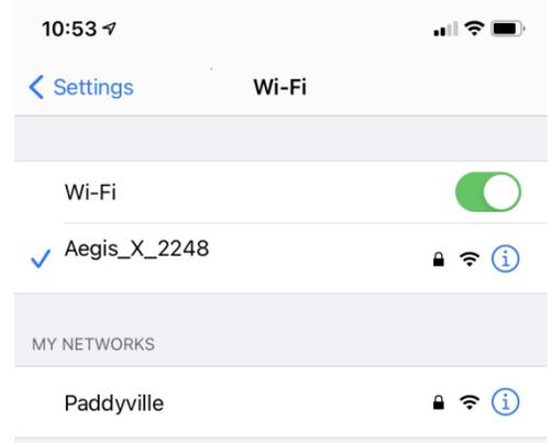
If there are more than one AegisX nearby, you will need to verify the controller by comparing the name with the last 4 digits of the serial number located on the side of the controller.
