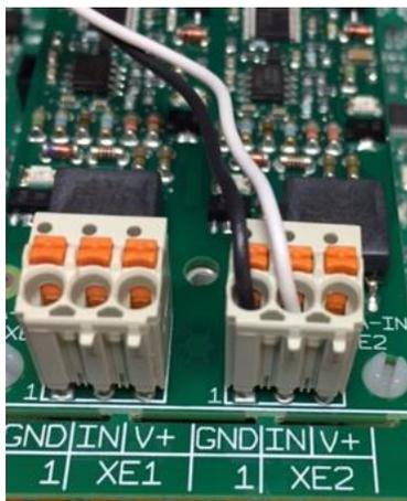
Milliamp inputs from powered devices do not need on-board V+. The + wire from the Input device, (analyzer, PLC, etc.), connects to the 'IN' terminal and the (-) wire to the 'GND'.
