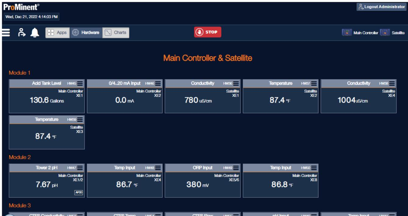
Here is an example of the top portion of the hardware page which shows analog signal boxes for the main and satellite enclosures. In this example, Module 1 shows the I/O of the module in the main unit (a dual 4-20mA Input card – 2 boxes) and the module in the satellite unit (a conductivity card – 2 conductivities and 2 temperature input boxes).
