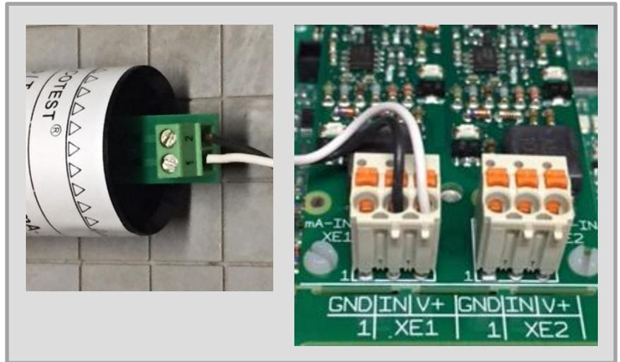
The above picture shows a ProMinent amperometric probe connected via a black and white wire to the XE1 terminal. White from pin 1 on the sensor to the V+ terminal and black from pin 2 to the IN terminal. The ground terminal on the module is not used for amperometric sensors.
