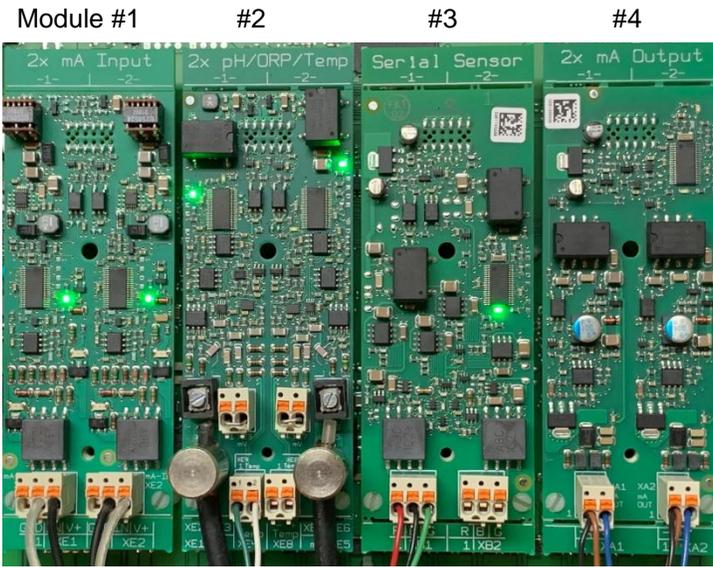
The dual analog output module can be set for 4/20mA or 0-20mA. Although somewhat rare, 0-20mA is still used. The advantage of 4-20mA is that you have a current representing a zero valve rather than no signal. A zero value signal happens when a wire is broken or is loosened from the termination point. This problem will not generate an error message when the 0 to 20 range is selected. A 4-20mA loop will alarm if the mA value is below approximately 3.8mA.
