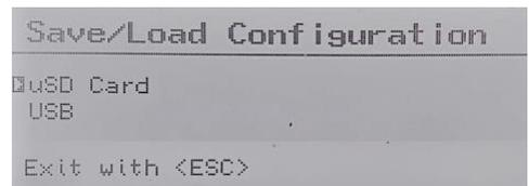
When loading a configuration, ensure that the driver cards in the controller are in the same slots as the new configuration. This includes the satellite slots. Load a configuration from an earlier saved version or from another controller (Cloning).
