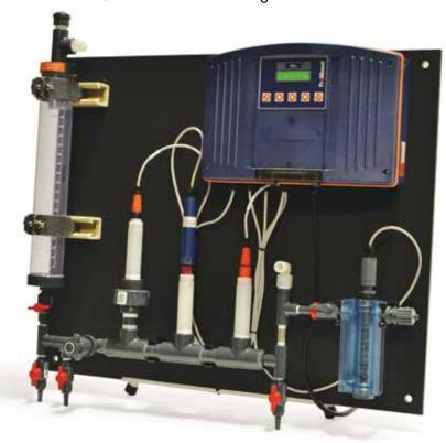
Continuous on-line measurement of ammonia using pH appropriate sensor technology. Uses specific sensor adapted to operational pH range to ensure correct measurement. Determine free ammonia, total ammonia, and NH<sub>3</sub>-N for control and reporting purposes. Complete system mounted on wall mountable backpanel to facilitate installation. Sample header includes ammonia sensor, pH sensor, and temperature sensor.
