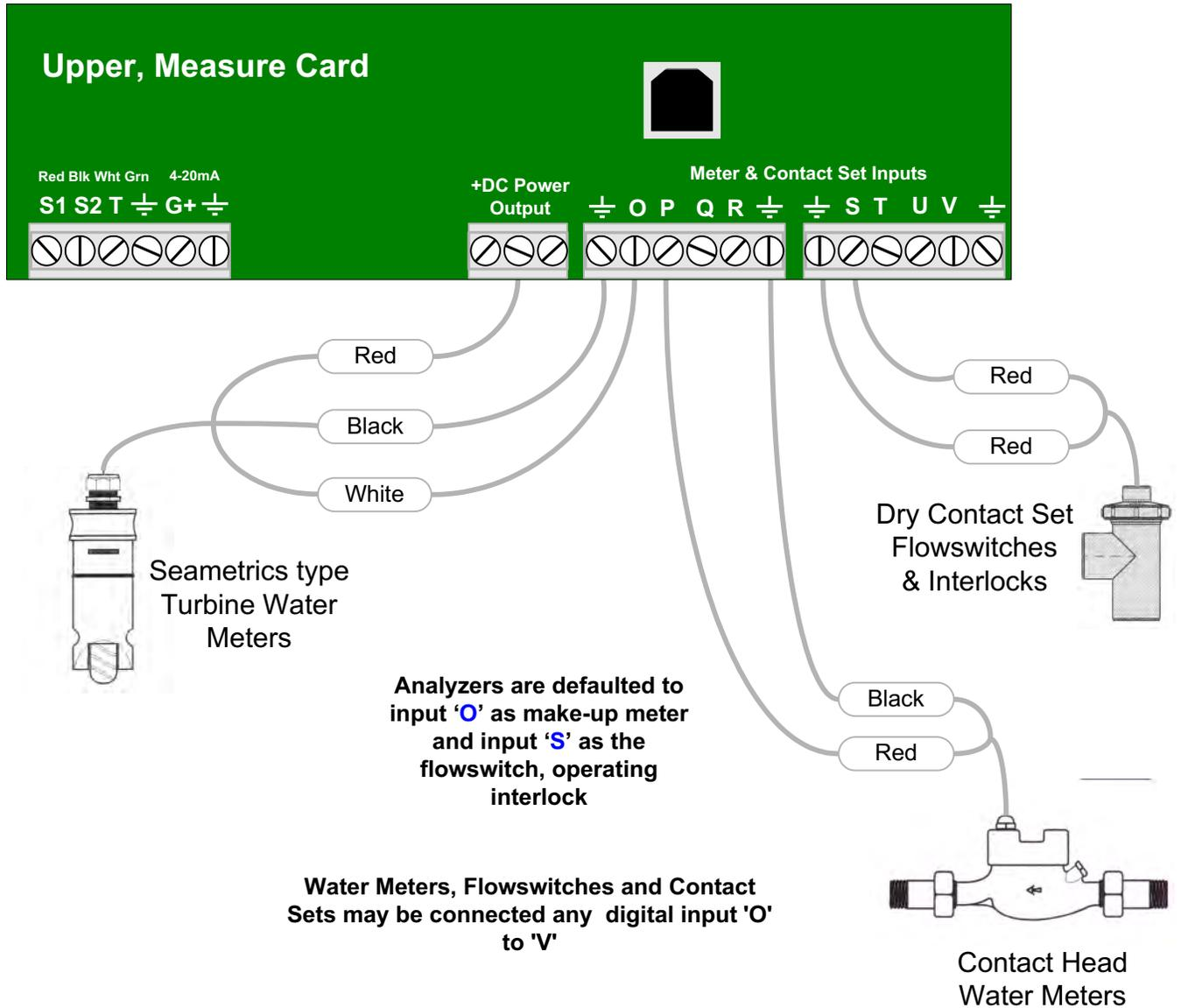
Connect cabling shields at the controller ends of the cable only, to any ground terminal either on the Measure card or on the aluminum backplate, bottom, center
