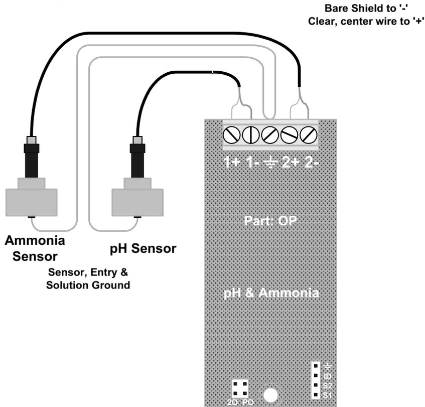
Do not install sensor cabling in the same conduit as AC power cabling.
