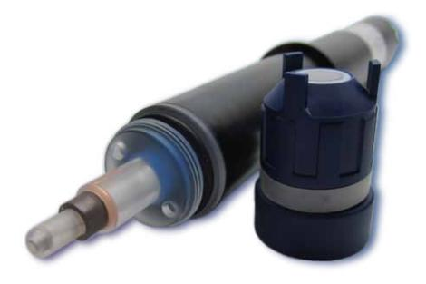
**ProMinent®** offers its new line of Free Chlorine sensors, the CBR series. These sensors were developed for measurement in water with higher pH, process water, cooling tower water, etc. The membrane covered Amperometric sensor measures both HOCI and OCI at pH values up to 9.5 without the need for buffers or reagents.
