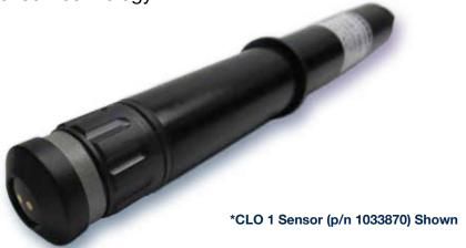
ProMinent® offers its new line of Free Chlorine sensors which offer membraneless technology in a reagentless medium. The CLO 1 and CLO 2 sensors offer precise measurement of free chlorine at temperatures up to 158° F and pressures to 116 psi. Each sensor has the capability to accurately measure free chlorine between a pH of 5-9.
