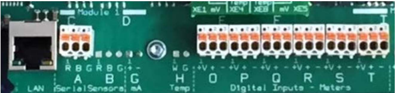
Figure 31 Main PC Board (Motherboard) inputs
