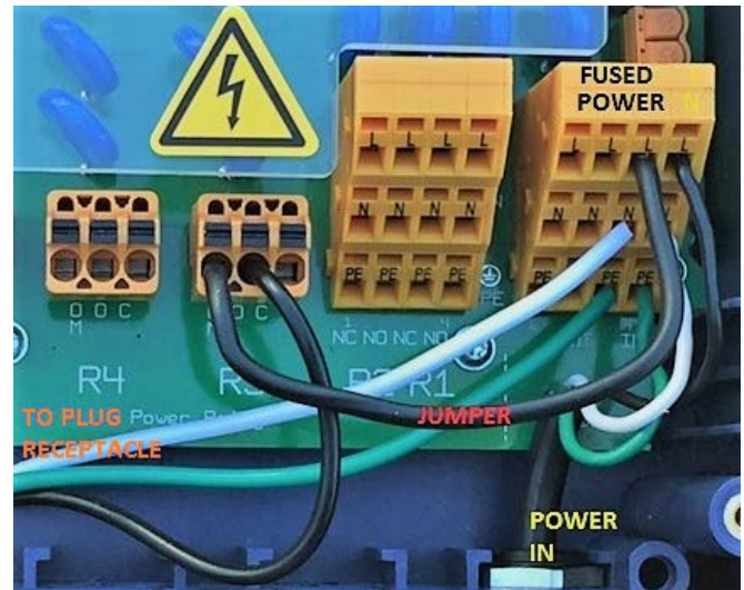
Figure 25 Wiring R3 using on-board fused power
