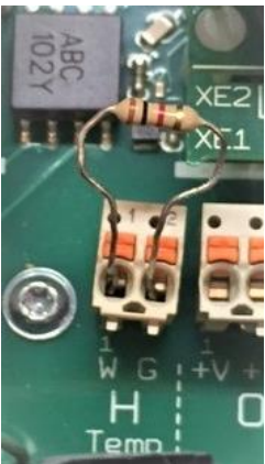
Figure 33 Input H with test resistor
