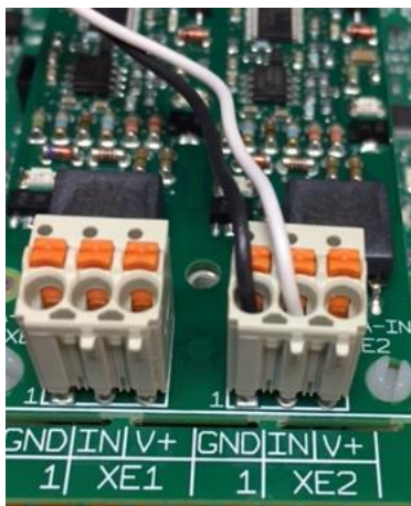
Figure 57 Two wire remotely powered analog input
