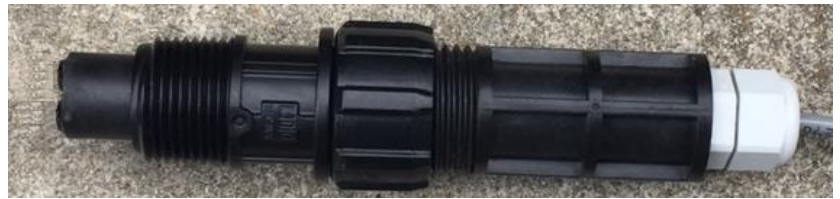
Figure 42 4 Wire Conductivity/Temperature sensor
