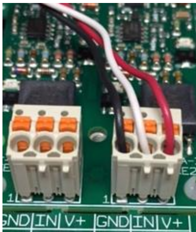
Figure 56 Three wire 4-20mA inputs that utilize V+
