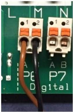
Figure 29D Universal Control Cable on Output Relay P6 (Enable/Disable-ON/OFF Mode)
