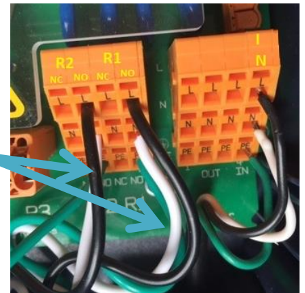
Figure 23 Terminating R1 & R2
