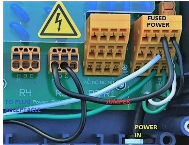
Figure 25 Wiring R3 using on-board fused power
