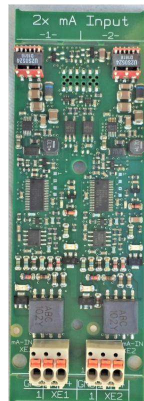
Figure 54 Dual 4-20mA Input driver
