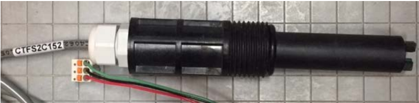
Figure 38B CTFS sensor shown without adapter
