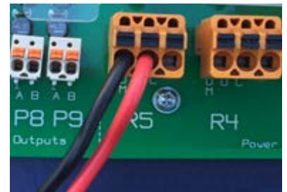
Figure 26 Remotely powered relay
