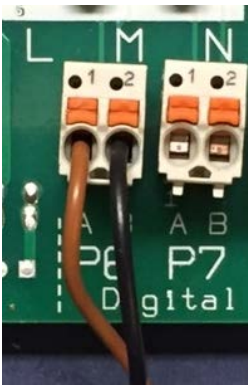
Figure 29E Concept pump cable on Output Relay P6 (Enable/Disable-ON/OFF Mode)
