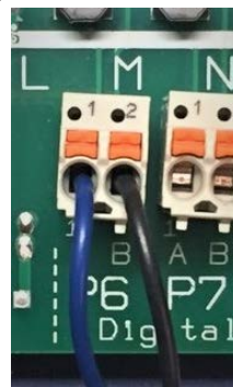
Figure 29C Concept pump cable on Output Relay P6 (Pulse Mode)
