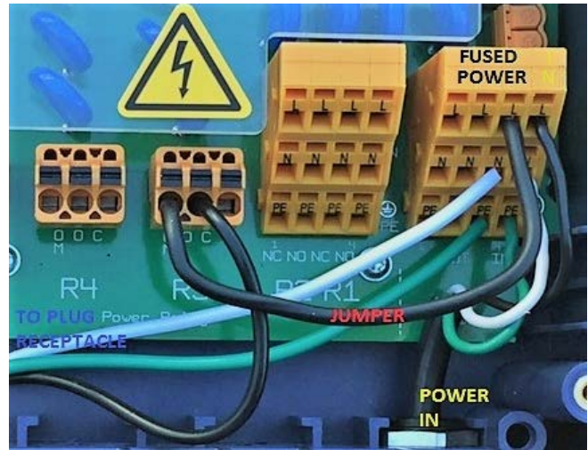
Figure 25 Wiring R3 using on-board fused power
