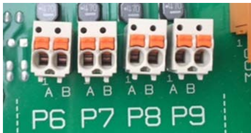
Figure 29A Digital DC outputs 6-9
