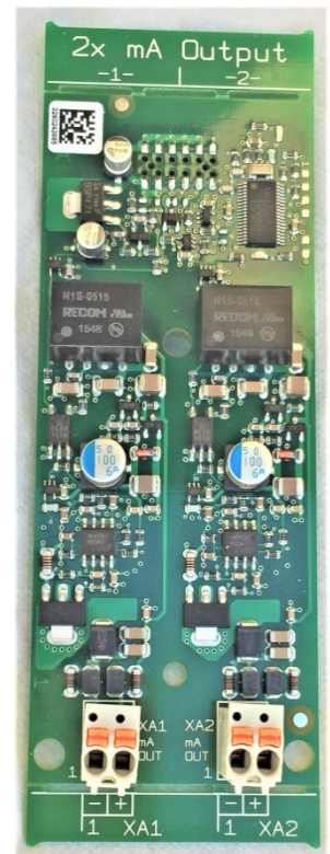
Figure 58 Dual 4-20mA Output driver
