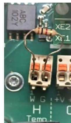
Figure 33 Input H with test resistor
